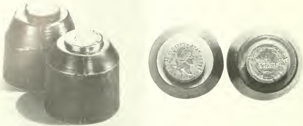
Fig. 85.—ORIGINAL DIES made by Robert Lovett in Philadelphia for the striking of Confederate cent, 1861.
