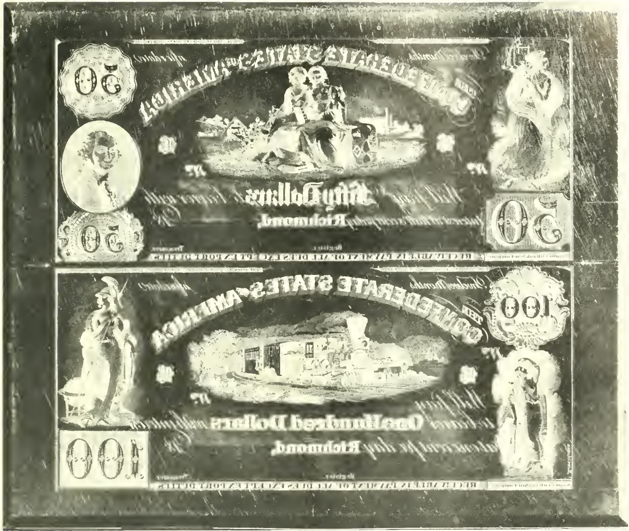
Fig. 67.—STEEL PLATE for the printing of Confederate 50-dollar and 100-dollar notes, 1861. Three quarters actual size.
