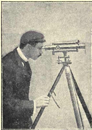
FIG. 129.—How NOT to use a level.
