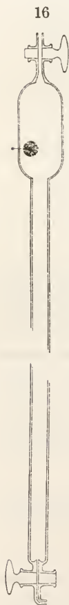
FIG. 16.—Tonometer electrode for determining the P_{\text{H}} of sea-water at a pre-determined \text{CO}_2 tension. A mixture of \text{CO}_2 and \text{H}_2 is bubbled through the sea-water in a narrow tube; then the stopcocks are closed and the electrode inverted so that the sea-water flows into the wide portion, which is of the same bore as the colorimeter tubes, so that the hydrogen electrode determination of the P_{\text{H}} may be compared with that by the colorimetric method. The stopcock on the wide end of the electrode is not greased, as it serves for electrolytic connection with the KCl bath.
