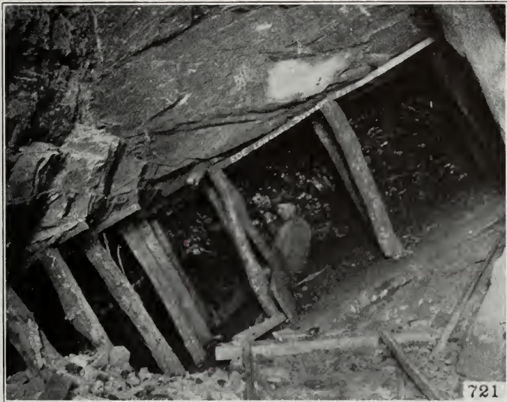
FIG. 25. Face of longwall panel mine in dipping seam (photo by H. I. Smith, U. S. Bureau of Mines)
