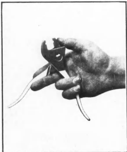
These pliers are instantly adjusted by moving the jaw with the thumb until the desired opening is reached
