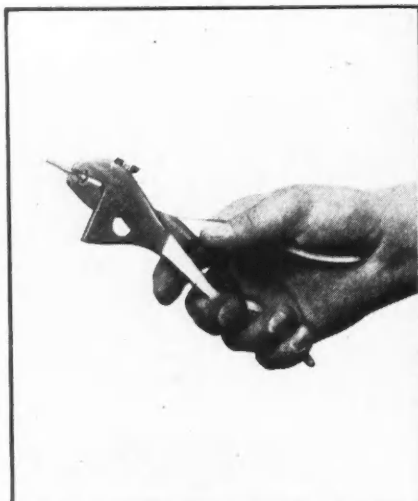
Through the leverage obtained by these pliers there is no danger of slipping in removing cotter pins
