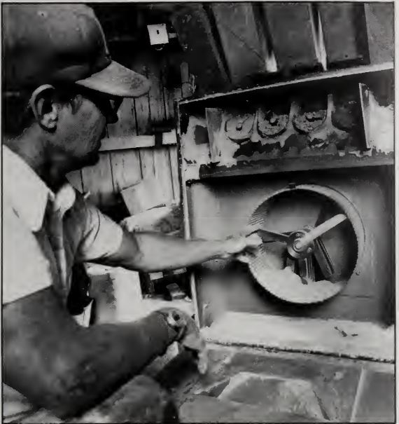
Carryover of medicated feed left in equipment can easily contaminate finishing feed.
