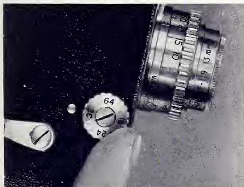
Any of four useful operating speeds, including "slow motion," may be used.
