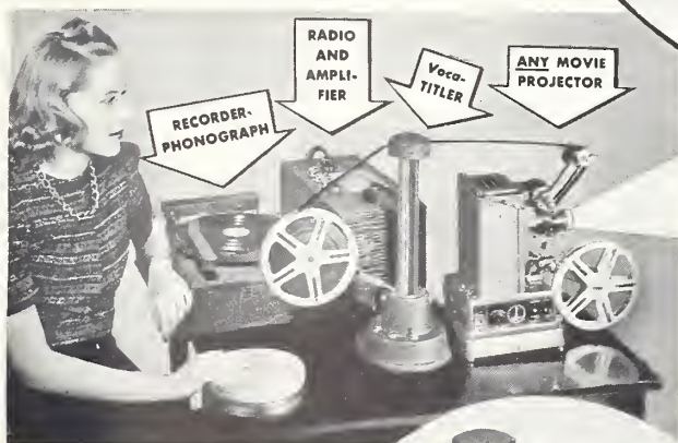
The Recorder-Microphone-Radio-Phonograph-Loudspeaker Unit (shown in upper circle) closes into an easy-to-carry case. Turntable runs at 78 r.p.m. and Recorder cuts 109 lines to the inch. About 30 titles of 20 words each can be put on either side of a 12-inch record. Included is 25-foot cable to Loudspeaker—$110. With Voca-Titler—$179.50.
