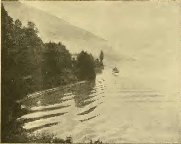
FIG. 1.—Wave-track of Steamer on Thunersee, showing thwart-ship and diverging waves. From "Waves of the Sea and other Water Waves."
