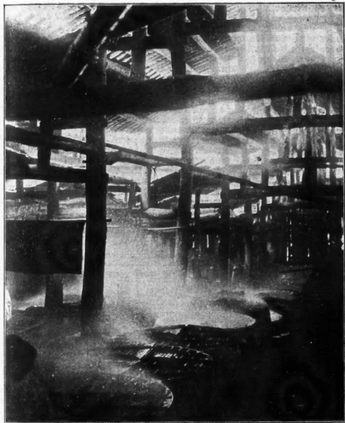
EVAPORATING SALT BY NATURAL GAS, CHINA.
