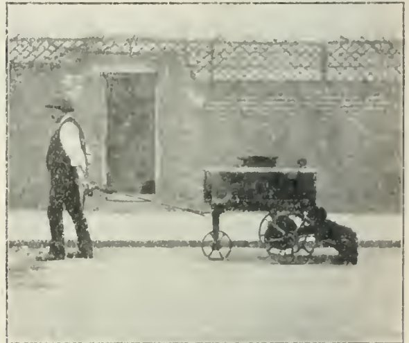
THE 50-GALLON HAND-DRAWN "FLAPPER" MACHINE.
