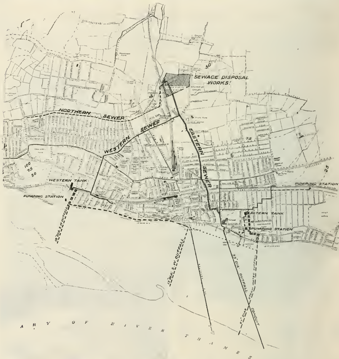
MAP SHOWING POSITIONS OF SEWAGE DISPOSAL WORKS, MAIN SEWERS, PUMPING STATIONS AND OUTFALLS, SOUTHEND-ON-SEA.
