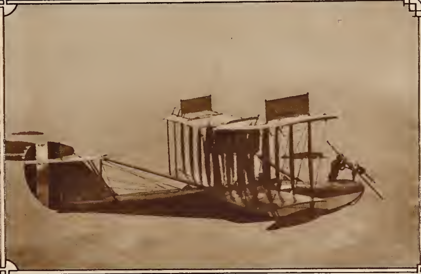
Navy hydroplane equipped with Davis non-recoil gun. In this gun the recoil force of the forward barrel is counterbalanced by that of a rear barrel from which a dummy charge is fired simultaneously with the projectile.
