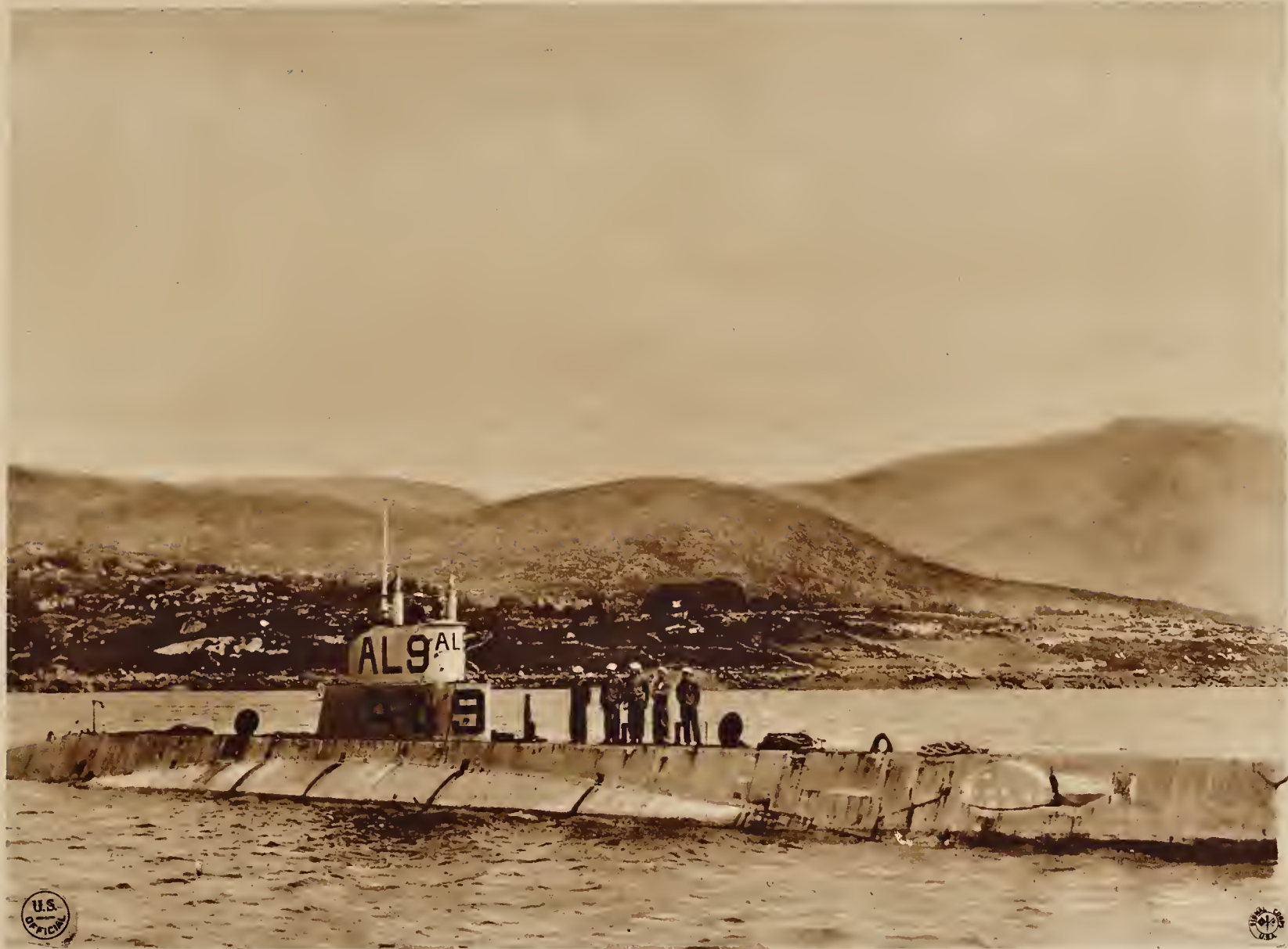
The A L 9 off the Irish Coast. "In the daytime Allied submarines remained under water, their periscopes exposed for a short time every fifteen minutes or so, sweeping the sea for a distance of many miles. As soon as darkness set in, the boats usually emerged, began taking in new air and recharging their batteries, the crews seizing the opportunity to stretch their legs and catch a welcome glimpse of the external world. 'We got used to your depth charges,' said the commander of a captured German submarine 'and did not fear them but we lived in constant dread of your submarines. We never knew what moment a torpedo was going to hit us.'" Rear Admiral Sims.
