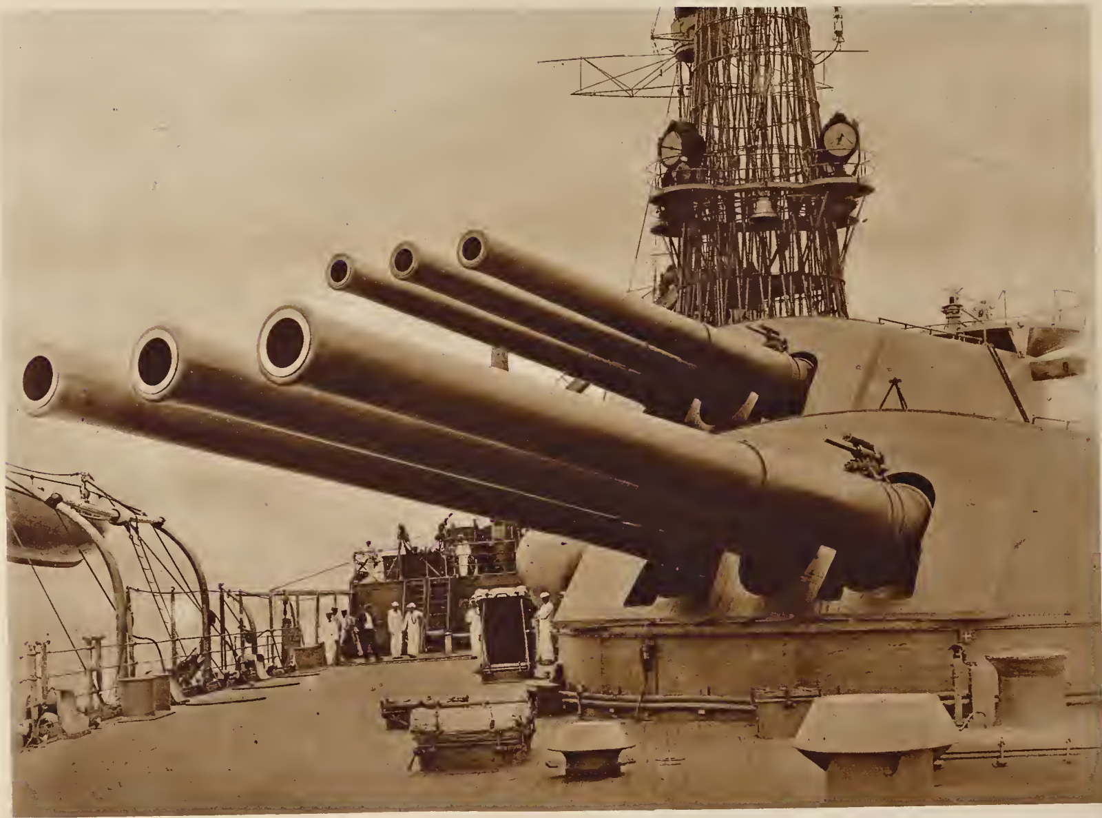
Guns of the U. S. S. "Pennsylvania," flagship of the Atlantic Fleet, Admiral Henry T. Mayo, Commander in Chief. The armament of the "Pennsylvania" consists of 12 14-inch, 45 caliber; 14 5-inch, 51 caliber; and 4 3-inch, 50 caliber guns and 2 21-inch torpedo tubes.
