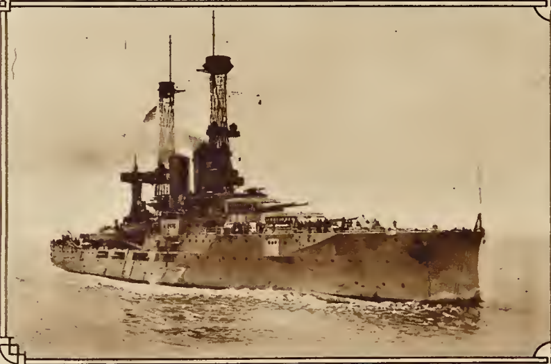
U. S. S. "Florida," commanded by Captain Thomas Washington, afterward Captain M. M. Taylor. Length 510 feet. Beam 88 feet 2½ inches. Draft 28 feet, 6 inches. Normal displacement 21,825 tons. Horse-power (main engine) 40,511. Trial speed 22.08 knots. Guns: 10 12-inch, 45 caliber; 6 5-inch, 51 caliber; 2 3-inch, 50 caliber A. A. Torpedo tubes (submerged) 2 21-inch. Photo from U. S. Navy. International Film
