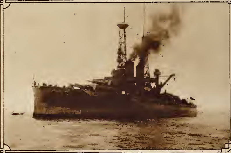
U. S. S. "Arkansas." Commanded by Captain W. H. G. Bullard, afterward Captain L. R. de Stiguer. The "Arkansas" relieved the "Delaware" July 30, 1918. Length 554 feet. Beam 93 feet 2½ inches. Mean draft 28 feet 6 inches. Normal displacement 26,000 tons. Horse-power (main engine) 28,533. Trial speed 21.05 knots. Guns: 12 12-inch, 50 caliber; 6 5-inch, 51 caliber; 2 3-inch, 50 caliber A. A. Torpedo tubes (submerged) 2 21-inch.
