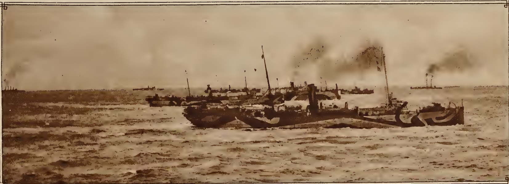
United States Mine Squadron in planting formation in the North Sea. On each of the thirteen operations there were eight ships in line abreast, with two in line abreast sailing ahead of them. The vessels were 500 yards apart. At the signal from the flag ship, "First Mine Over," the mine layers, going at full speed, would drop mines at intervals of fifteen seconds for three or four hours. According to Rear Admiral Sims there were four planters which on several "excursions" lay about 860 mines in 3 hours and 35 minutes in a single line about 44 miles long. These were the Canandaigua, the Canonicus, the Housatonic, and the Roanoke.
