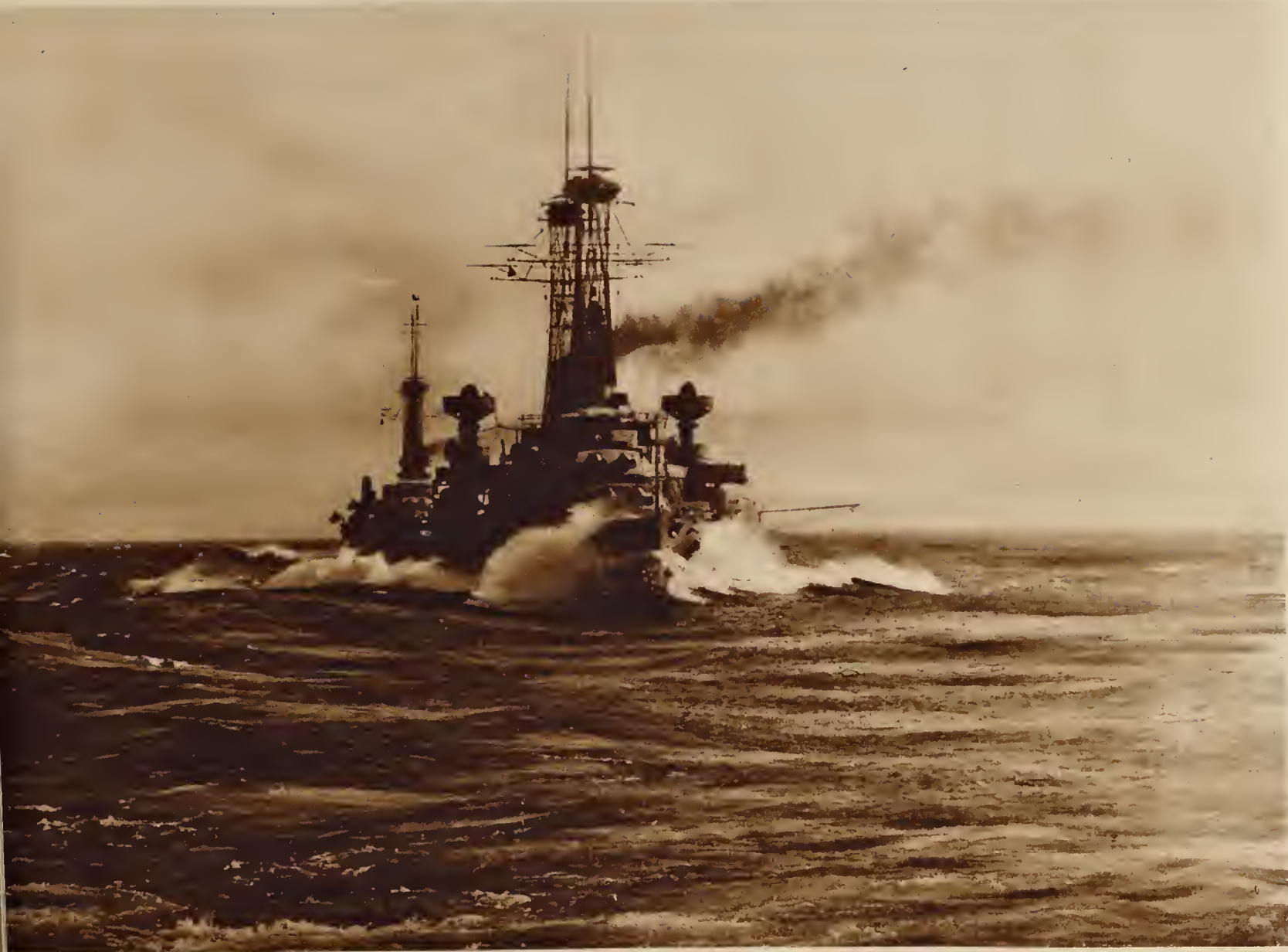
The Sixth Battle Squadron in column. Leading is the U. S. S. "New York," which was commanded by Captain C. F. Hughes, afterward Captain E. L. Beach. Length 565 feet. Beam 95 feet, 2½ inches. Mean draft 28 feet, 6 inches. Normal displacement 27,000 tons. Horse-power (main engine) 29,687. Trial speed 21.47 knots. Guns: 10 14-inch, 45 caliber; 6 5-inch, 51 caliber; 2 3-inch, 50 caliber A. A. Torpedo tubes (submerged) 4 21-inch.
