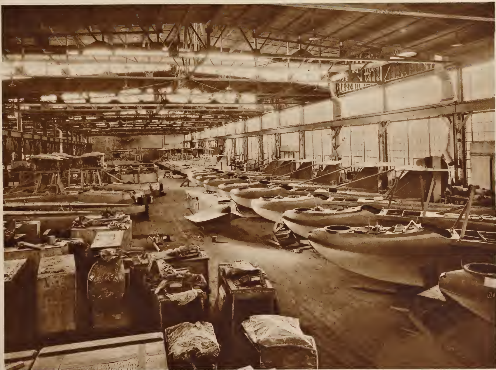
HS-1-L final assembly floor at the North Elmwood Plant of the Curtiss Aeroplane and Motor Corporation, Buffalo, N. Y. Nov. 11, 1918.
