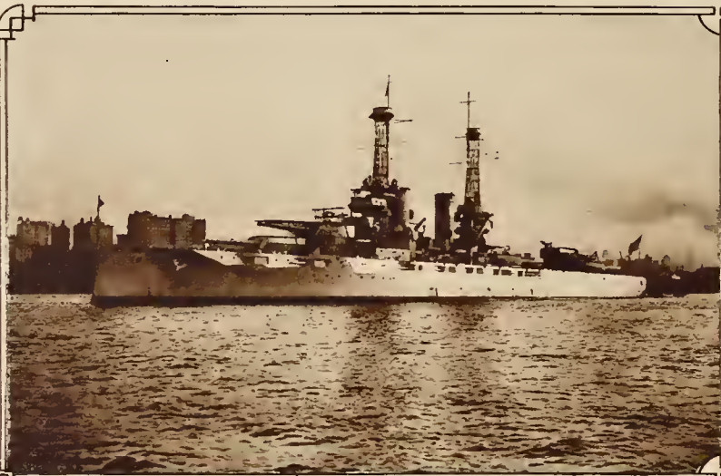
U. S. S. "Texas." Commanded by Captain Victor Blue. Length 565 feet. Beam 95 feet 2½ inches. Mean draft 28 feet 6 inches. Normal displacement 27,000 tons. Horse-power (main engine) 28,373. Trial Speed 21.05 knots. Guns: 10 14-inch, 45 caliber; 6 5-inch, 51 caliber; 2 3-inch, 50 caliber A. A. Torpedo tubes (submerged) 4 21-inch. Photo from U. S. Navy.
