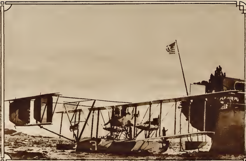
Warming up the motors of NC-3 at Trepassey through steam-pipes of U. S. S. "Prairie."
