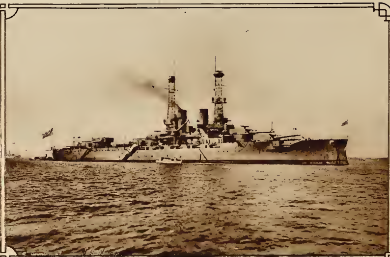
U. S. S. "Wyoming," commanded by Captain H. A. Wiley, afterward Captain H. H. Christy. Length 554 feet. Beam 93 feet 2½ inches. Mean draft 28 feet, 6 inches. Normal displacement 26,000 tons. Horse-power (main engine) 31,437. Trial speed 21.22 knots. Guns: 12 12-inch, 50 caliber; 6 5-inch 51 caliber; 4 3-inch 50 caliber A. A. Torpedo tubes (submerged) 2 21-inch. Photo from U. S. Navy.
