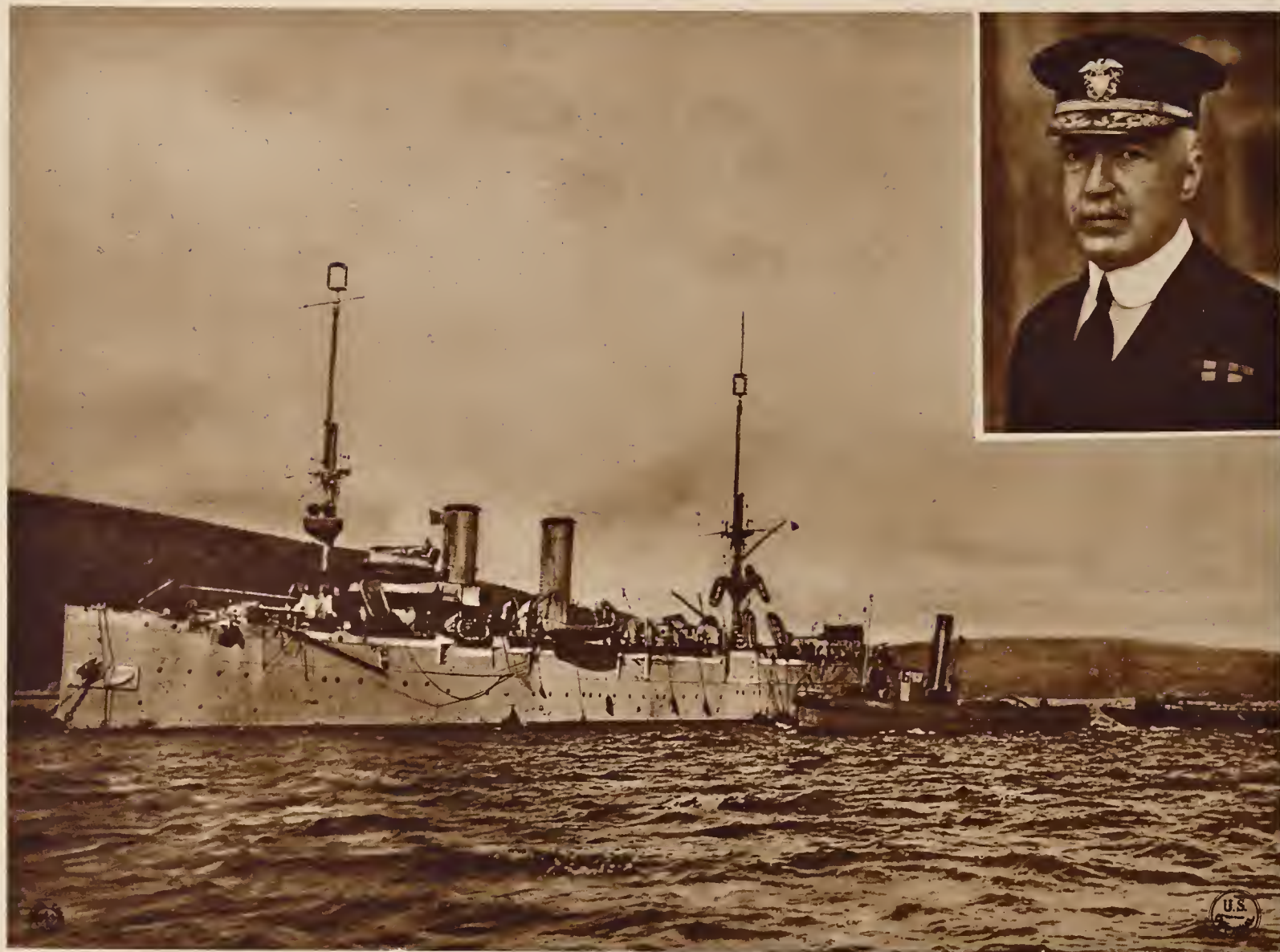
U. S. S. "San Francisco," flagship of Minelaying Squadron One at Inverness. The tug is bringing a lighter laden with mines alongside. The length of the "San Francisco" is 310 feet. Beam, 49 feet 2 inches. Mean draft, 18 feet 9 inches. Mean displacement, 4,093 tons. Trial speed, 19.52 knots. Guns: Four 5-inch, 51 caliber; two 1-pounders. Inset—Rear Admiral Joseph Strauss who took command of the minelaying operations in March, 1918.
