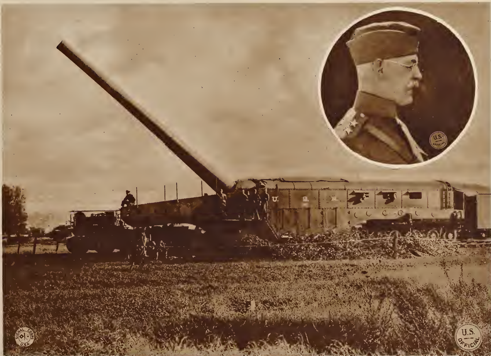
SILENCING THE BIG BERTHA. Five naval 14-inch guns on railway mounts constructed by the Baldwin Locomotive Works were landed in St. Nazaire in July, 1918. They were under the command of Rear-Admiral C. P. Plunkett, U. S. N. Their main mission, says Admiral Sims, was to destroy the "Big Bertha" which was raining shells on Paris and to attack strong points, especially railroad communications, and the bridges across the Rhine. Admiral Sims adds: "Expertly as this unusual train had been camouflaged, the German airplane observers had detected its approach. As it neared the objective, the shells that had been falling on Paris, ceased; before the Americans could get to work the Germans had removed their mighty weapon, leaving nothing but an emplacement as a target for our shells. Though our men were therefore deprived of the privilege of destroying this famous long range rifle, it is apparent that their arrival saved Paris from further bombardment, for nothing was heard of the gun for the rest of the war." Up to the Armistice the guns fired 782 shells at distances ranging from 18 to 23 miles. They played havoc in the railroad yards at Laon, Montmedy and Conflans. Inset: Rear Admiral C. P. Plunkett, U. S. N.
