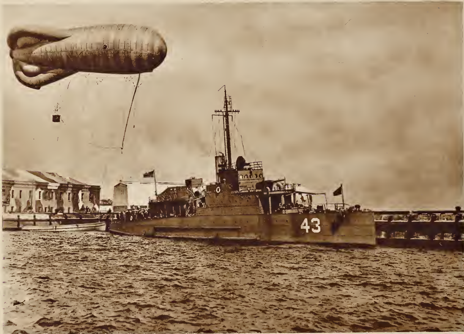
Navy observation balloon at Pensacola, Fla. In the middle ground of the picture is Ford Eagle boat No. 43. In the last days of 1917 Henry Ford of Detroit agreed to undertake the construction of anti-submarine patrol boats and to place the whole energy of his enormous force and organization behind the work. The first Eagle was completed and given a successful trial on Lake Huron, Oct. 10, 1918. The second Eagle was placed in commission Nov. 8, 1918, and the third a few days later. Sixty boats were made for the Navy, of which five were transferred to the Treasury Department for Coast Guard duty. The length of these boats between perpendiculars is 200 feet. The width of beam on load water line is 25 feet 6 inches. The mean draft is 7 feet 3 inches and normal displacement is 500 tons. The type of engine is the Poole geared turbine. There are 2 Bureau express oil burning boilers. The trial speed of Eagle No. 1 was 18.32 knots. The mess complement is: 5 ward room officers, 4 chief petty officers and 52 men.
