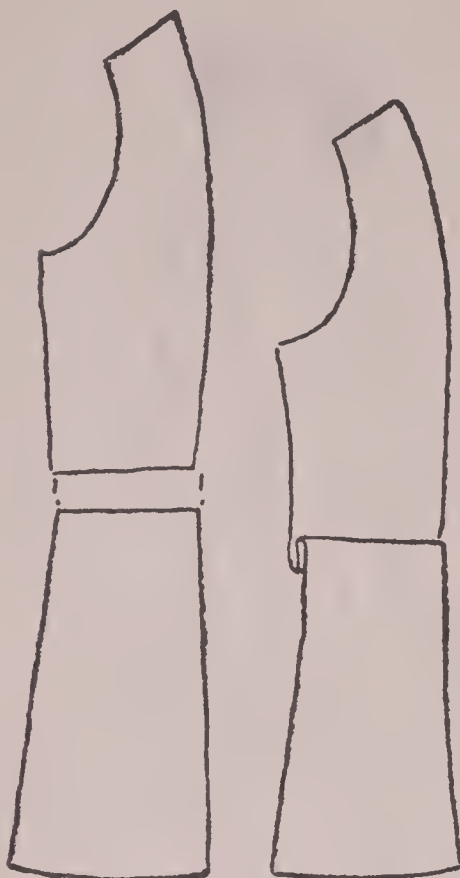
Fig. (43) Making the coat pattern longer waisted Fig. (44) Making the coat pattern shorter waisted
