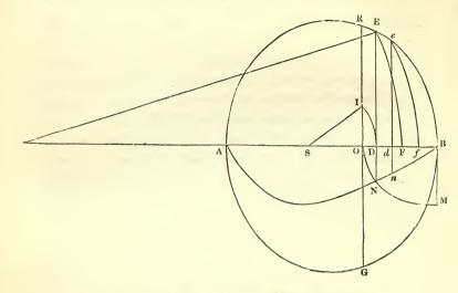
(=u) equal to P.S.  $r^{n-1}$   $y^2$ , and let B.D=z, and the curve B.N.A will be described, and the differential area N.D.d.n will be ndz= (by construction) P.S.  $r^{n-1}$   $y^2$  dx; consequently u dz will be the attractive force of the differential solid E e f F; and  $\int u \, dz$  will be that of the whole body or sphere A.E.B, therefore the area A.N.B= $\int u \, dz$  is equal to the whole attraction of the sphere.
