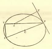
circle, and joining V F, which is, therefore, parallel to Y P, we have V P : P F :: S Y : S P or C : 2 R :: p : r and  $C = \frac{2 R \cdot p}{r}$ , which substituted for C in the above
