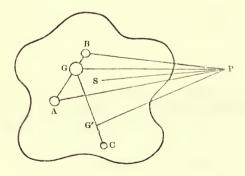
$G P \times A = A P \times G$ , therefore the forces in the line A P destroy each other, and there remain only  $P G \times B$  and  $P G \times A$  to draw P, that is  $(A + B) \times P G$ ; and the same may be shown of any other particles C and the
