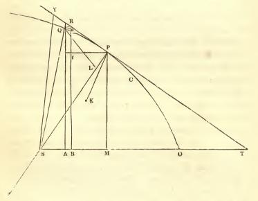
the last expression; and, therefore, Q R being parallel to LP, the central force at P is as  $\frac{Q R}{S P^2 \times L Q^2}$ . So if S Y be the perpendicular upon the tangent P Y, because P R and the arc P Q, evanescent, coincide, twice the triangle S P Q is equal to S Y × Q P; and the
