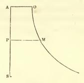
force at P in terms of A P or x, or the gravitation of any particle of a homogeneous fluid towards S at the point P; then the column of that fluid whose altitude is A P will press at P, as the area A P M O, or as  $v^2$ , the square of the velocity acquired by a body falling through A P.
