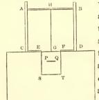
will be greater than the weight of a cone whose base is PQ and altitude HG, and less than that of a spheroid on the same base and of the same altitude. For let HP and HQ be the boundaries of the cataract. The cataract falls freely, and therefore there is no pressure on the sides of the mass of still
