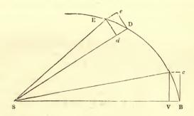
B C and D E the arcs described in a given time; C c and E e lines parallel to the radii vectores S B and S D respectively; and C V, E d parallel to the tangents. The centripetal forces at B and D must be in the proportion of V B and d D (being the other sides of the parallelograms of forces) if the arcs are evanescent, so as to coincide with the diagonals of the parallelograms V c and d e. Hence the centripetal forces in B and D are as the versed sines
