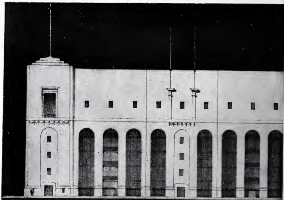
Exterior Elevation of a south tower and a portion of the adjoining wall according to the final scheme of continuous, open and exposed expansion joints.
