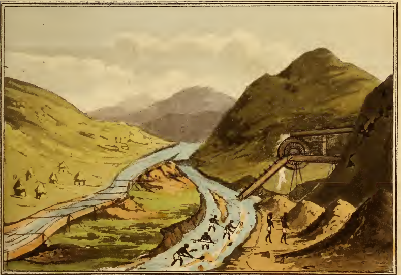
BED OF THE RIVER LAID DRY BY AN ACQUEDUCT, TO COLLECT THE ALLUVIAL SOIL, IN ORDER TO WASH IT FOR DIAMONDS, GOLD, &c.
