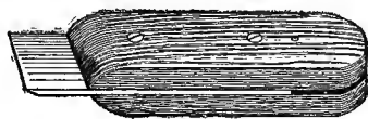
FIG. 104.—Knife for freezing microtome, made from the blade of a carpenter's plane.
