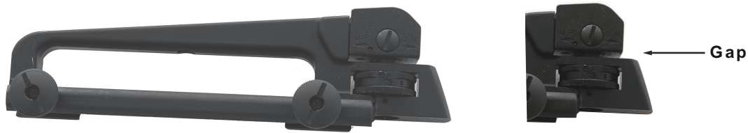
Figure 8-16. Rear Sight Elevation Knob Set for 600 Meters/Yards.
