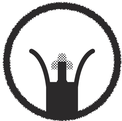
Figure 5-8. Correct Sight Picture with Iron Sights.
