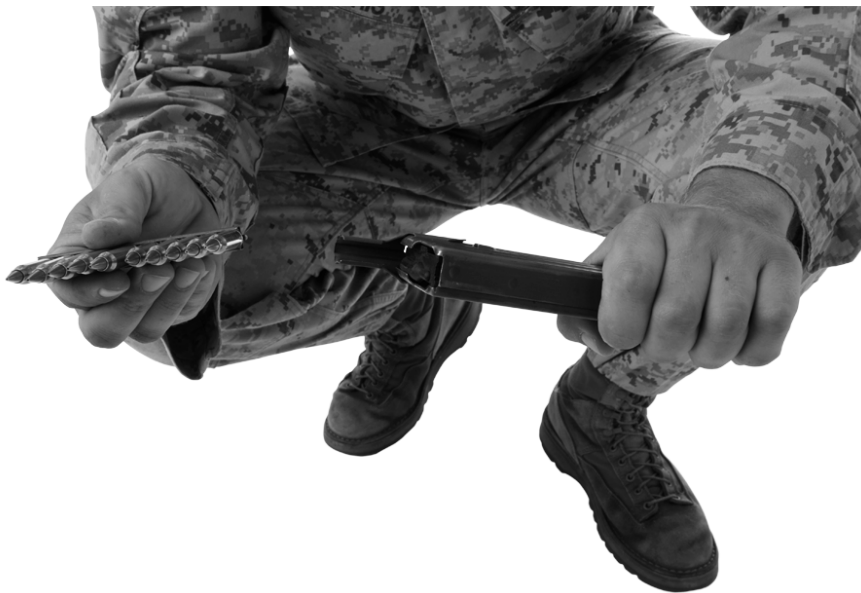
Figure 4-9. Filling the Magazine with a Stripper Clip and Magazine Filler.
