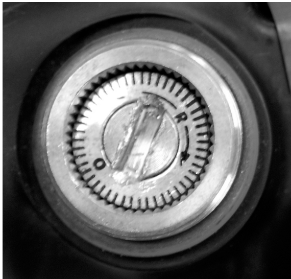
Figure 8-3. Service Rifle Combat Optic Windage Adjuster.
