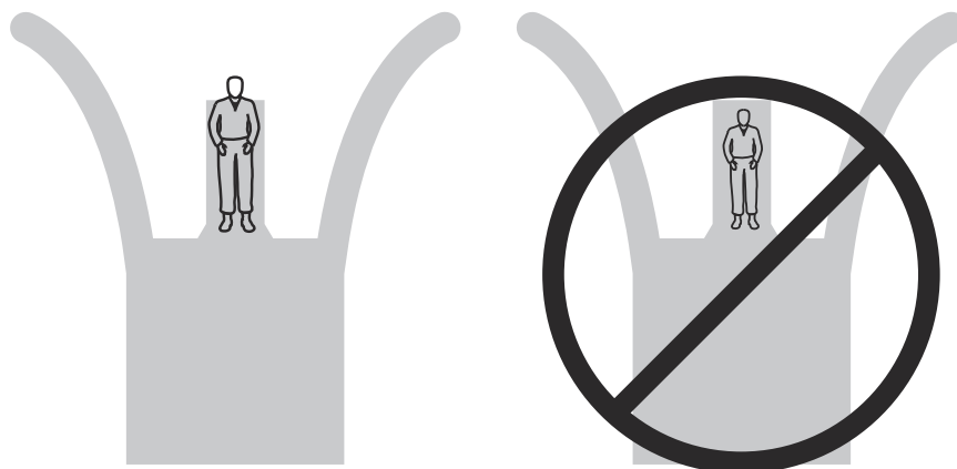
Figure 9-9. Offset Aiming Points for Elevation Outside Battlesight Zero.
