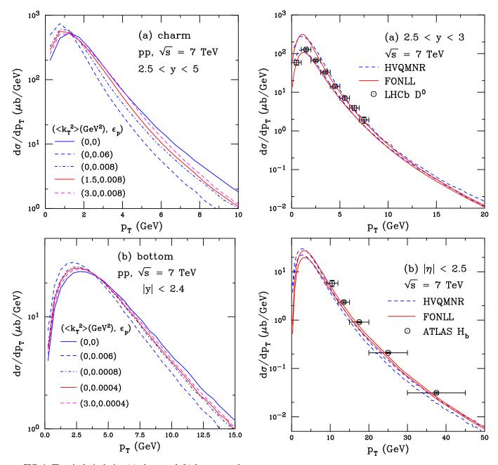
FIG. 4. The single inclusive (a) charm and (b) bottom quark distributions in  $\sqrt{s}=7\,\mathrm{TeV}~p+p$  collisions at next-to-leading order using the HVQMNR code. The charm distributions are given at forward rapidity, 2.5 < y < 5, while the bottom quark distributions are given at midrapidity, |y|<2.4. Results are shown for various combinations of  $\langle k_T^2 \rangle$  [Eq. (3)] and  $\epsilon_P$  [Eq. (4)].
