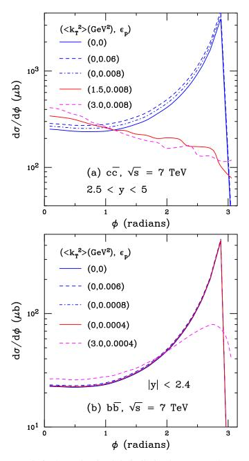
FIG. 6. The NLO azimuthal distribution between two heavy quarks,  $d\sigma/d\phi$  in p+p collisions at  $\sqrt{s}=7$  TeV using the HVQMNR code for (a)  $c\overline{c}$  pairs at forward rapidity, 2.5 < y < 5, and (b)  $b\overline{b}$  pairs at midrapidity, |y| < 2.4. The results are shown for the same combinations of  $\langle k_T^2 \rangle$  in Eq. (3) and  $\epsilon_P$  in Eq. (4) as in Fig. 4.
