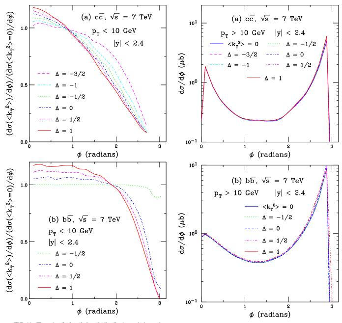
FIG. 11. The ratio of azimuthal angle distributions relative to that of  $\langle k_T^2 \rangle = 0$  for (a)  $c\bar{c}$  and (b)  $b\bar{b}$  pairs in the central rapidity range |y| < 2.4 with  $p_T < 10$  GeV. Calculations are shown for values of  $\Delta$  from -3/2 to 1 for charm and  $\Delta = -1/2$  to 1 for bottom, as in Eq. (9).
