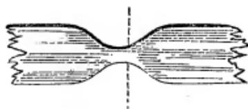
*To mend a Test-tube.*—Test-tubes frequently for a moment to fuse the sharp edges.
