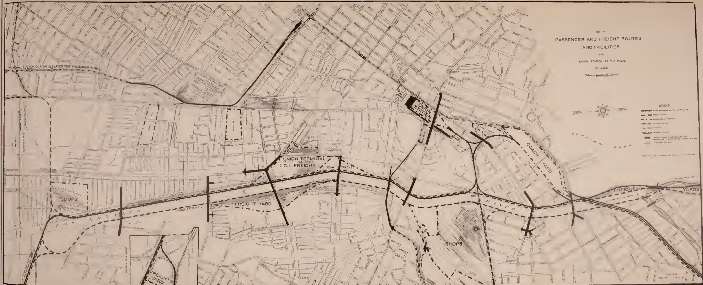
FIG. 130 ROUTE MAP WITH UNION STATION AT THE PLAZA This plan has been made by the Engineering Department to show the location of passenger and freight routes and facilities as recommended. The passenger routes from the north and from Pasadena will pass to the west of the freight yards and trackage. Those from the east will reach the station directly along Alhambra Avenue, and those from the south will run adjacent to the river on a new double track bridge. Through freight will use the east bank of the river.
