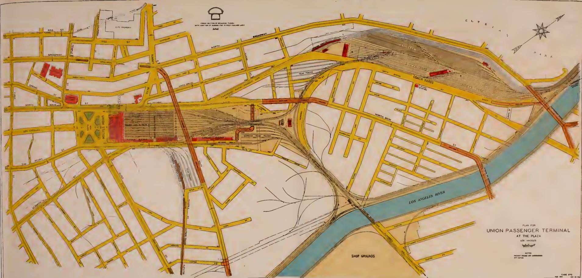
FIG. 129. ENGINEERING DEPARTMENT PLAN FOR A UNION PASSENGER TERMINAL AT THE PLAZA. This plan as it would be developed twenty or thirty years hence is shown. Note the convenient relation of the station to the coach yard and shop grounds, the strategic location of the station building near the end of the built up business district, and the accessibility and general convenience of the site.
