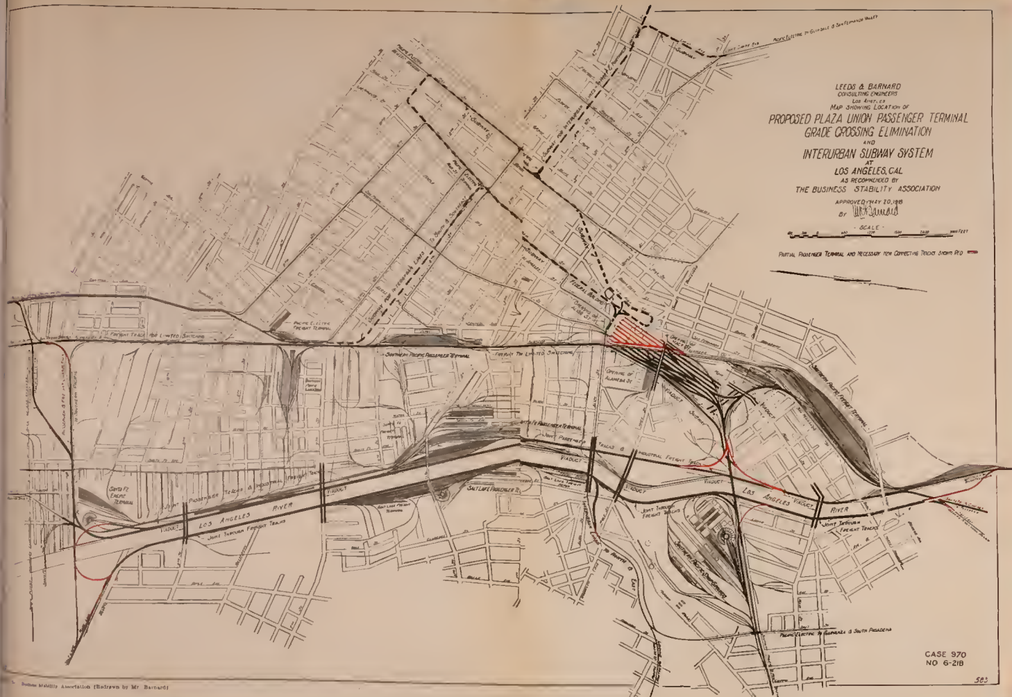
FIG. 111. BARNARD PLAN FOR UNION PASSENGER TERMINAL AT THE PLAZA This is the plan recommended by the Business Stability Association. This plan and the recommended Engineering Department plan makes use of the same site. Proposed immediate construction is shown in red
