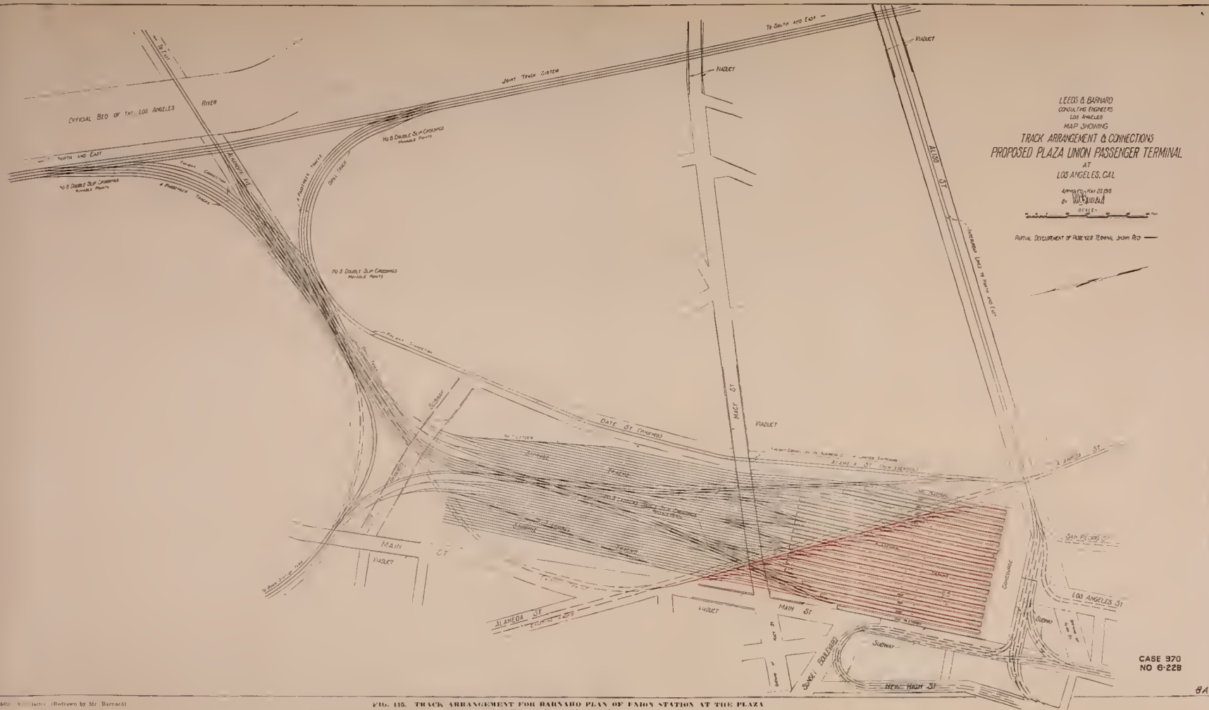
FIG. 116. TRACK ARRANGEMENT FOR BARNARD PLAN OF FAIR STATION AT THE PLAZA The ultimate plan is shown and consists of 11 tracks. The tracks are depressed below the level of the Plaza to the level of Alameda Street
