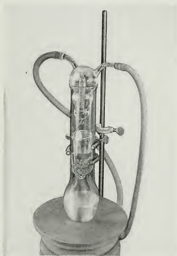
Fig. 2.—Apparatus for extracting non-rubber components from GR-S.
