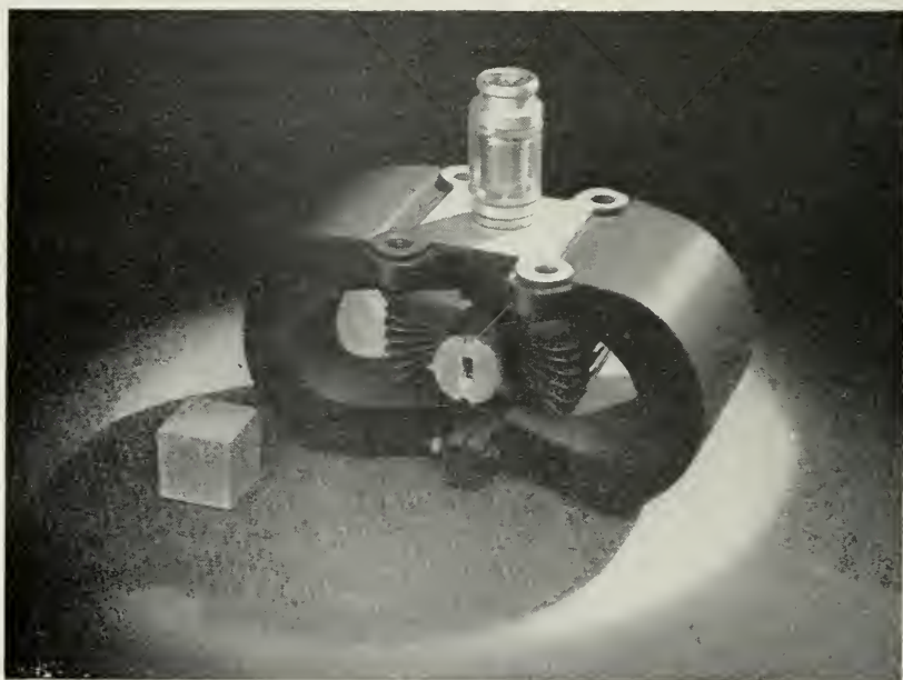
Fig. 76—An external view of the 3J21 “packaged” magnetron (60 kw., 24,000 mc/s).
