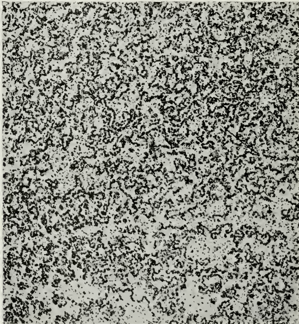
Fig. 15—Photomicrograph ( \times 15 ) of a section through a sintered iron sponge showing porosity.
