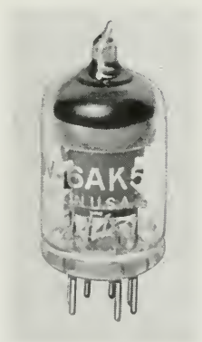
Fig. 3—Western Electric 6AK5 vacuum tube (full size).
