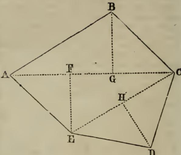
And in the same manner, a field of six, seven, or eight sides, may be divided into triangles by measuring lines across it; but to those unacquainted with land surveying, it would be best to take, if a ploughed field, a number of ridges at a time, and find their content by some of the first rules; then take more ridges and find their content also, until all the ridges are taken, and the summing up of the whole will be the content of the field.
