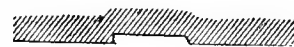
Details of the groove cut on each side of the course A. HORIZONTAL SECTION.
