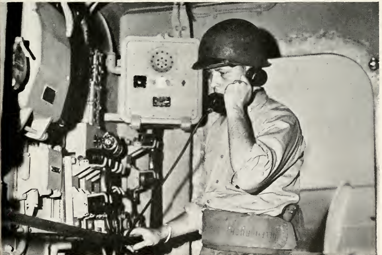
A SOUND-POWERED TELEPHONE in use aboard a U. S. warship
