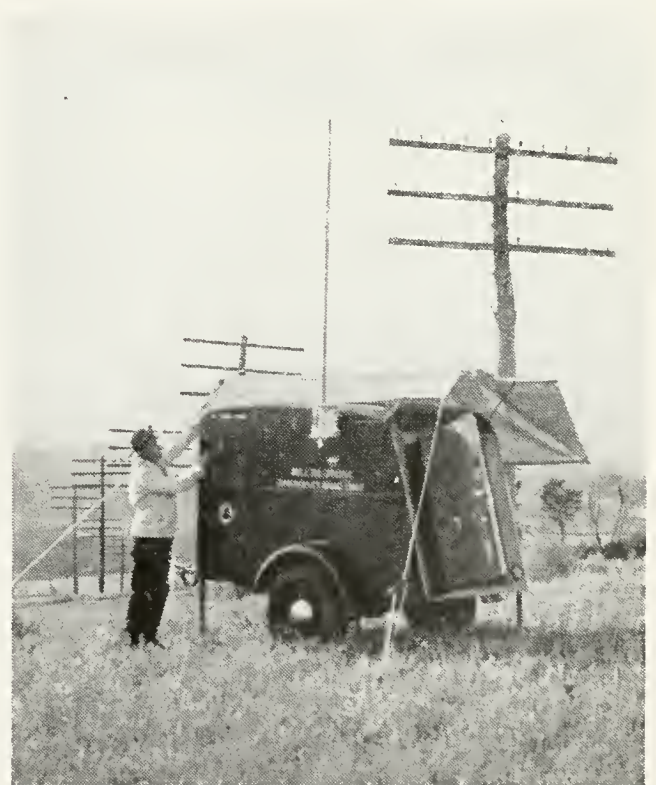
An emergency radio telephone station. A pair of these compact stations can bridge a temporary gap in physical circuits to handle two-way conversations
