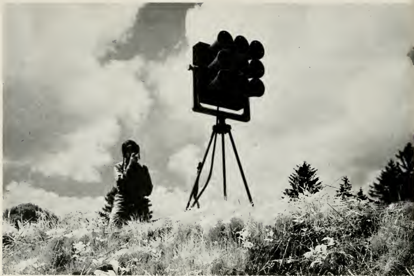
TRAFFIC COP OF INVASION: the Laboratories' "beachmaster" adaptation of a Bell System public address loudspeaker (above). Truck-mounted rocket launchers (below) in action using a fire-control device developed by the Laboratories
