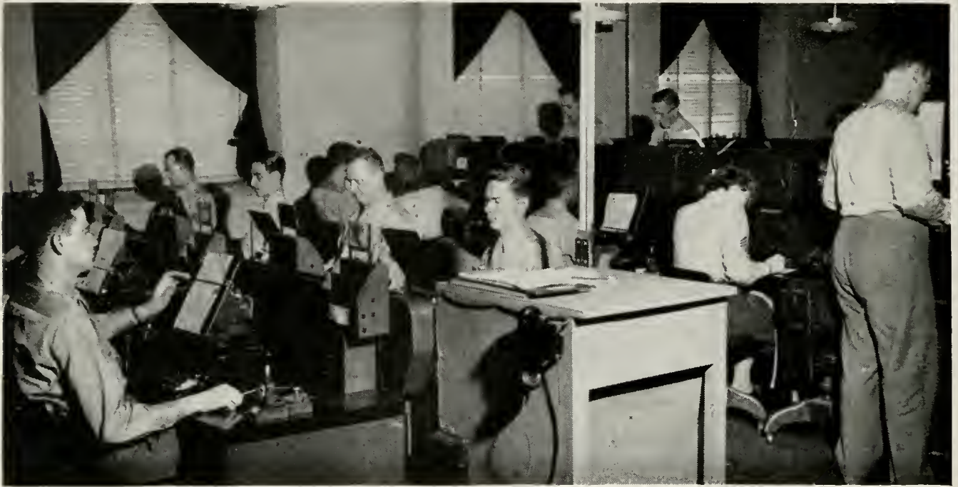
Station W A R, Washington. In this section of the Signal Corps' message center, messages are being punched on tapes for automatic transmission
