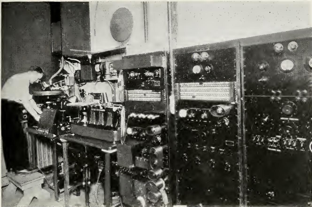
"Cutting a disc" in 1926. The apparatus at the left is engraving sound vibrations on a wax disc, duplicates from which will be played in synchronism with a film
