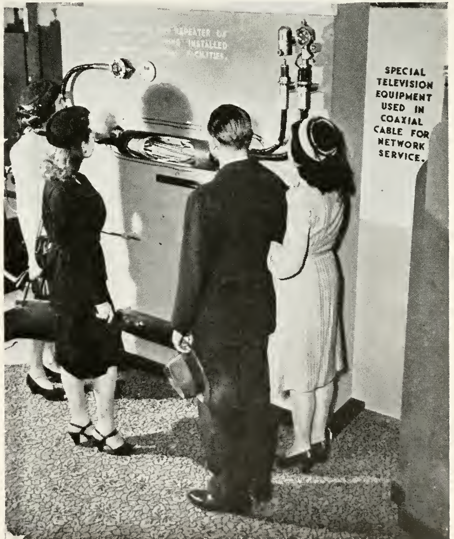
A cutaway section of a coaxial cable splice, and a repeater and a gas pressure gauge, were included in the Bell System's exhibit of television equipment
