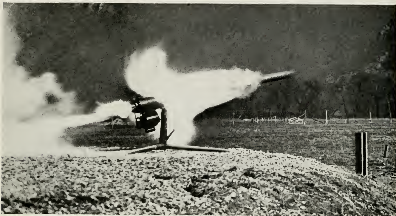
A ROCKET starts its journey, its accuracy increased by the spin imparted in launching
