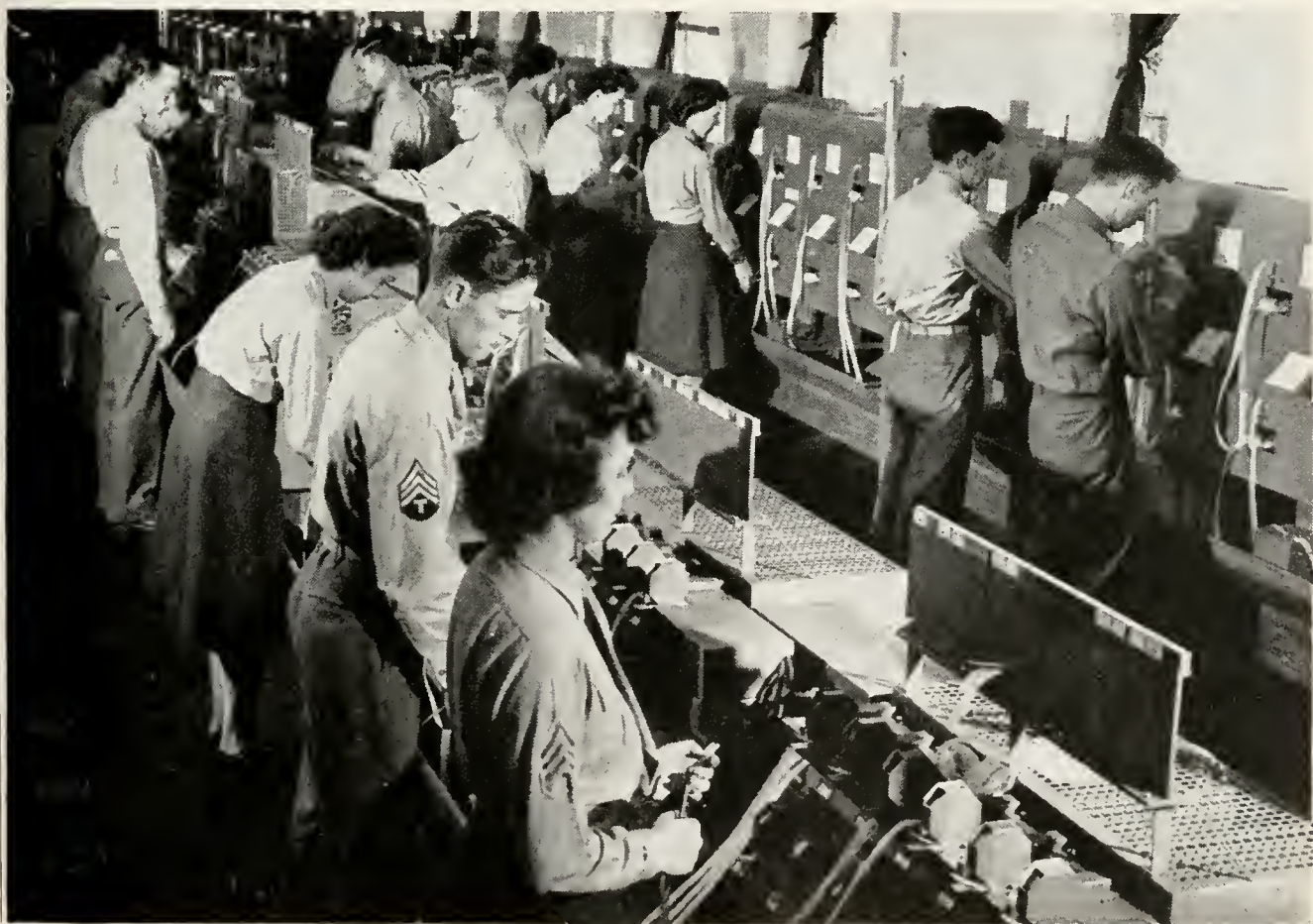
Here Signal Corps personnel are attending the automatic transmitting (foreground) and receiving machines
