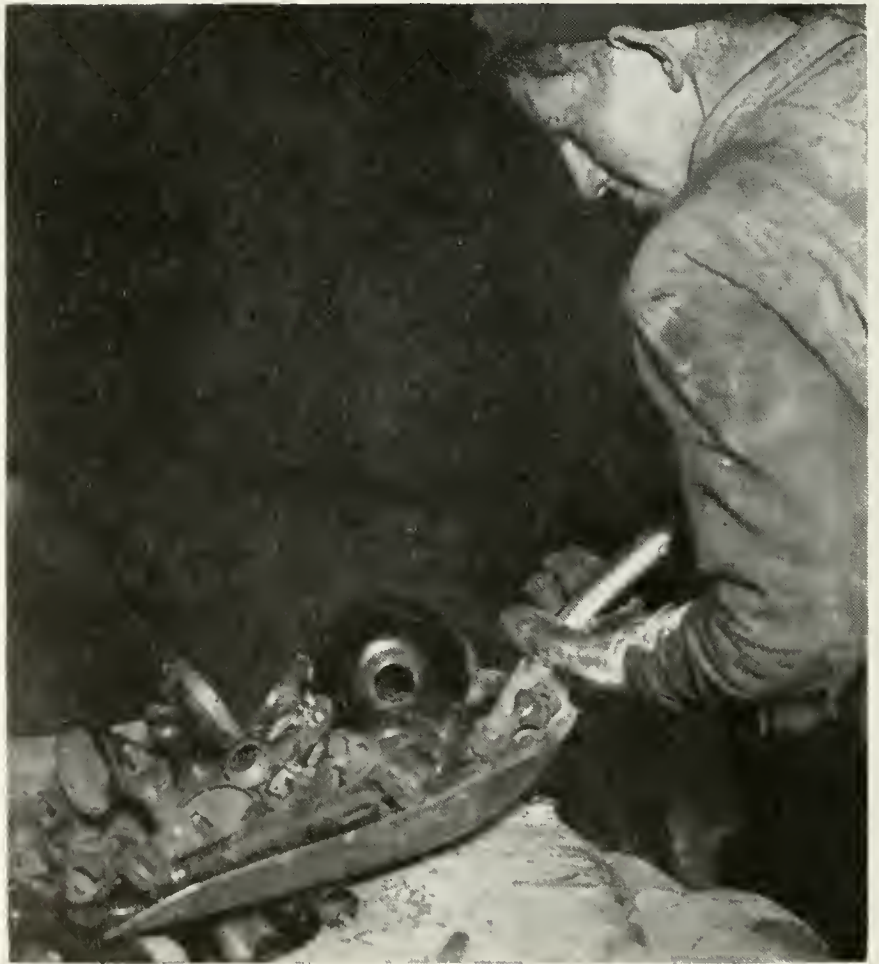
Into the furnace go these remnants of worn out telephones, and out will come brass billets
