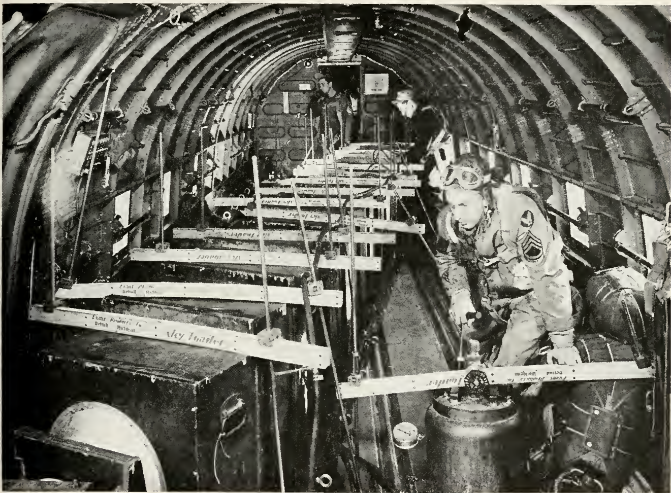
SIXTEEN MILES of field wire are coiled within the boxes fastened securely in this plane, the outside end of each coil spliced to the inside end of the next coil
