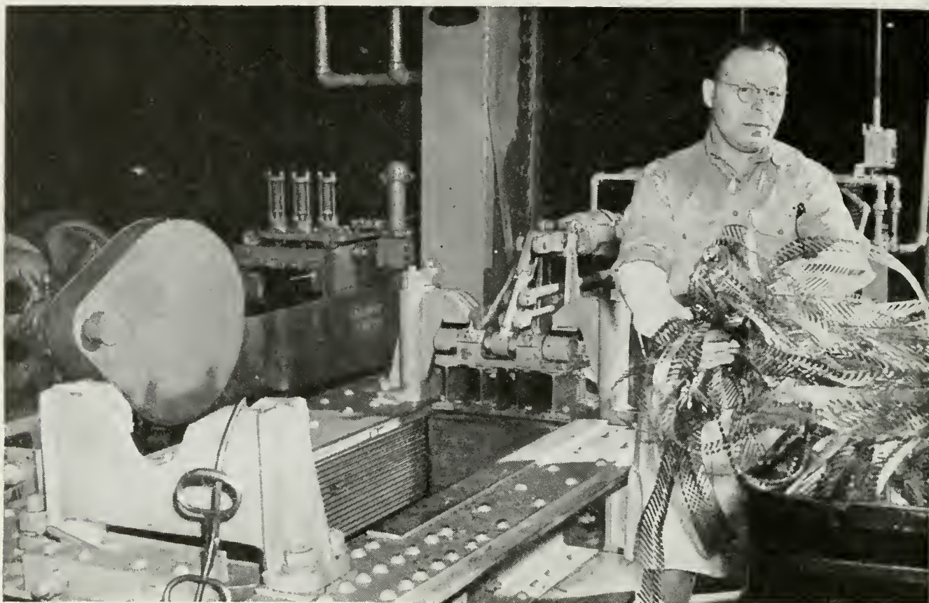
An operator in the reclamation department of one of Western Electric's Works loads scrap metal into a baling machine. The Nassau company supervises the reclamation and disposal of all scrap material throughout the Bell System
