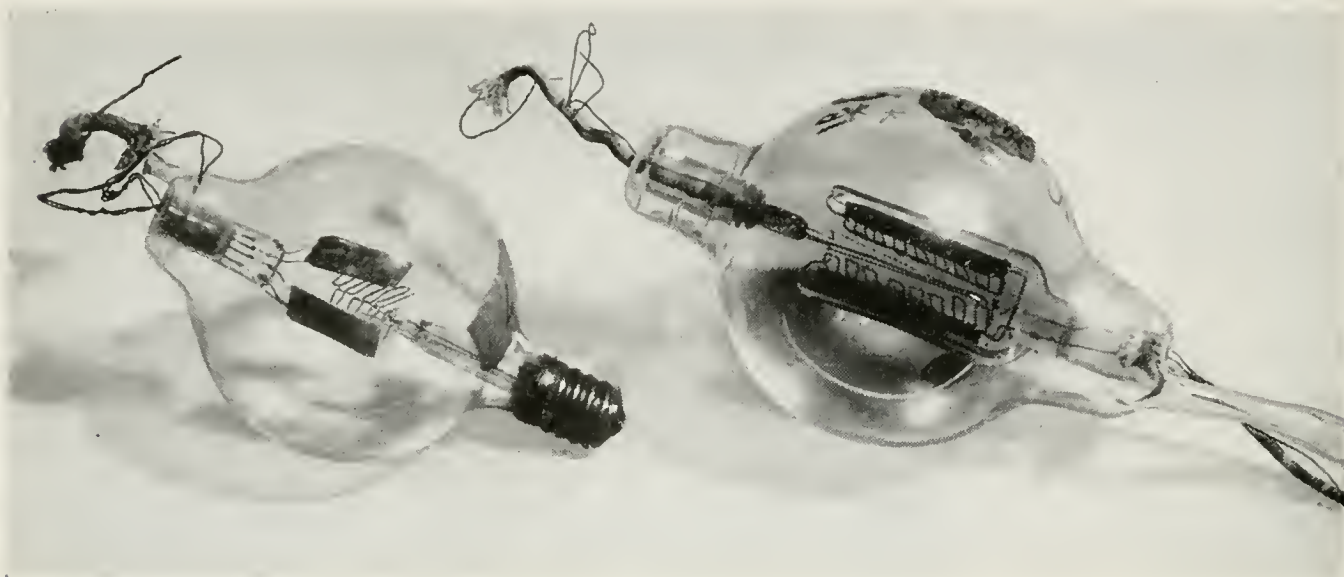
DeForest's audion as submitted to Dr. Jewett in 1912 (left), and the high-vacuum tube developed in 1913 for the first telephone repeater
