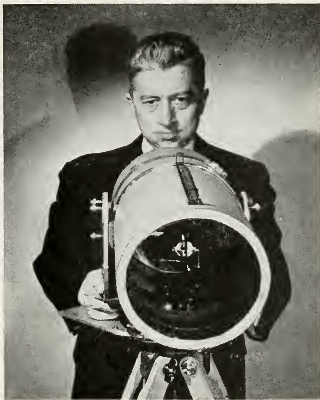
A thermistor bolometer, useful in measuring minute changes in temperature
