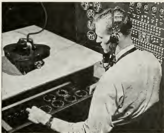
The flight instructor can create conditions within the trainer which simulate those found aloft
