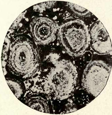
FIG. 92a. — Oolitic phosphate, Cokeville, Wyo. \times 30 .
