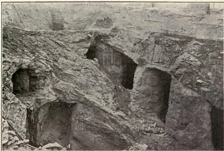
FIG. 1. — View of open cut in magnetite deposit, Mineville, N. Y. The pillars are left to support the gneiss hanging wall. (After Witherbee, Iron Age, Dec. 17, 1903. )
