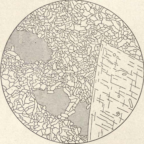
FIG. 225. — Photo-micrograph of jasperoid, showing fine granular aggregate of quartz, with sphalerite (shaded) and dolomite, the latter including minute quartz crystals. \times 53 . (After Smith and Siebenthal.)
