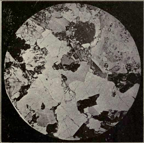
FIG. 52.—Photomicrograph of a section of Granite. (Photo loaned by A. B. Cushman.)
