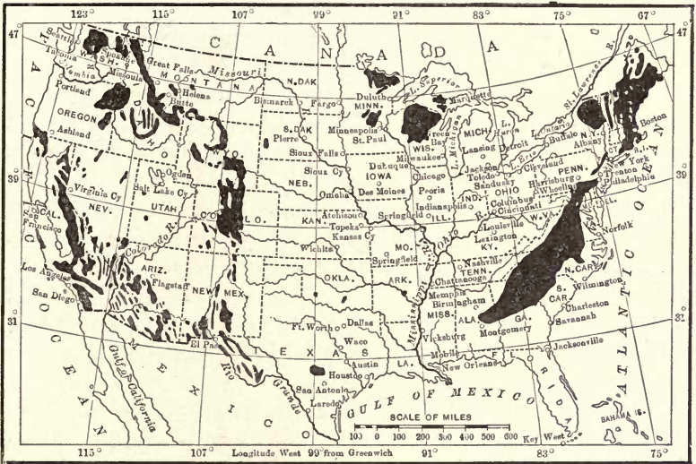
FIG. 55. — Map showing distribution of crystalline rocks (mainly granites) in United States. (After Merrill, Stones for Building and Decoration .)
