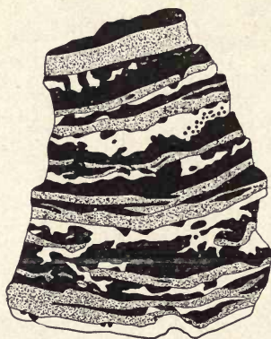
FIG. 127. — Banded sulphur-bearing rocks from Sicily; black, sulphur; dotted, limestone; white, calcite. (From Stutzer, Die Nicht-Erze .)
