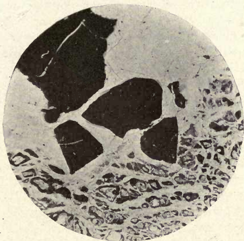
FIG. 135. — Chromite in olivine (in part altered to serpentine), from Kraubath, Austria. \times 15 .
