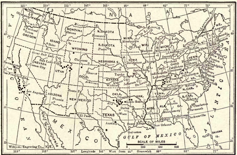
Fig. 46. — Map of asphalt and bituminous rock deposits of the United States. (After Eldridge, U. S. Geol. Surv., 22d Ann. Rept., IX.)
