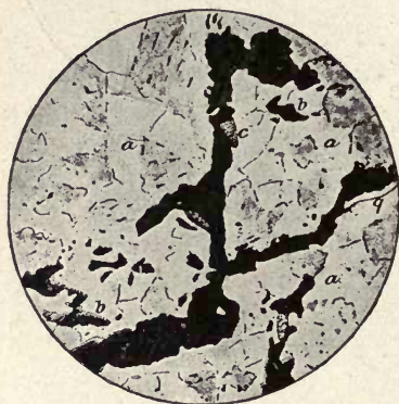
FIG. 141. — Replacement vein in syenite rock, War Eagle Mine, Rossland, B.C. (a) granular orthoclase with a little sericite; (b) secondary biotite; (q) secondary quartz; (c) chlorite; black, secondary pyrrhotite. (After Lindgren, Amer. Inst. Min. Engrs., Trans. XXX.)
