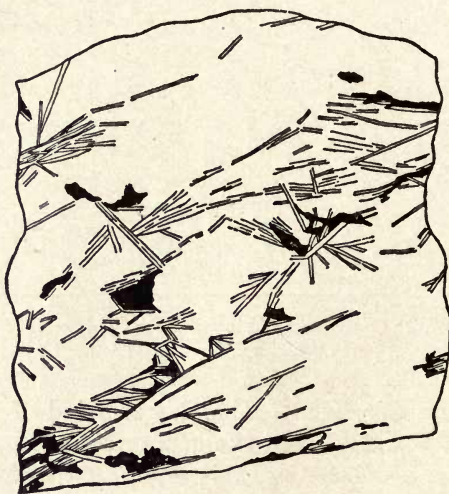
FIG. 211. — Section of ore from Chestnut Yard, Va., showing pyrrhotite (white) and chalcopyrite (black) replacements in hornblende (parallel lines). (After Weed and Watson, Econ. Geol. , I.)
