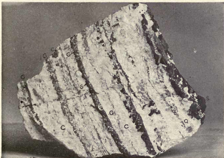
FIG. 2.—Banded vein, same locality. Sphalerite, S ; Galena, G ; Chalcopryite, C (black); Calcite, C (white); streak of later quartz, Q .
