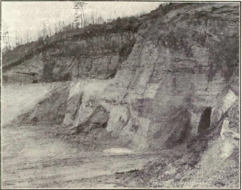
FIG. 1.—View in glass sand pit, on Severn River, Md.—The tunnel shows position of bed of glass sand. The overlying beds carry too much iron oxide. ( H. Ries, photo. )
