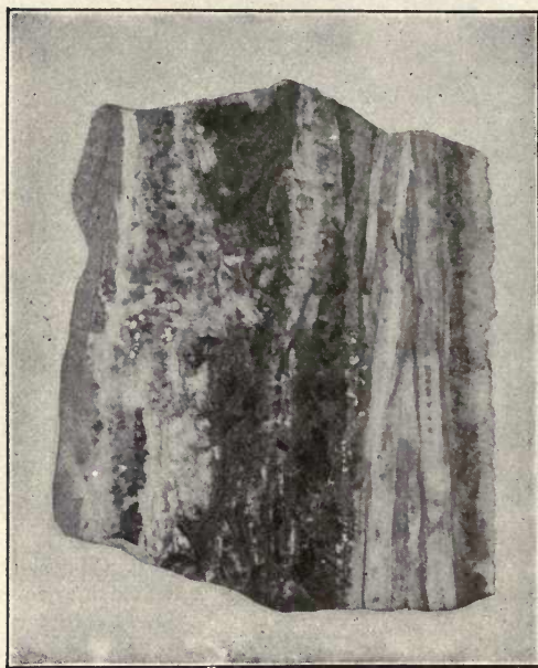
FIG. 144. — Section of vein in Enterprise mine, Rico, Colo. The right side shows later banding due to reopening of the fissure. (After Ransome, U. S. Geol. Surv., 22d Ann. Rept., II.)
