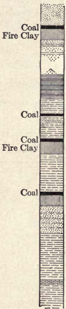
FIG. 2. — Section in coal measures of western Pennsylvania, showing fire clay under coal beds. (After Hopkins.)
