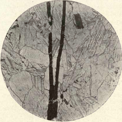
FIG. 195.—Thin section of crystalline limestone containing branched veinlet of sulphides, from Phoenix, B. C. \times 33 .
