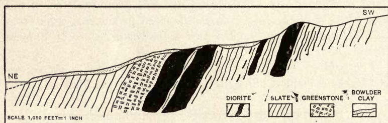
FIG. 243. — Cross section through Alaska Treadwell mine on northern side of Douglas' Island. (After Spencer, U. S. Geol. Surv., Bull. 259.)
