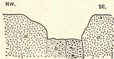
FIG. 280. — Section of Brown's chromic iron ore mine, Shasta County, Calif. a , Pyroxenite, in some places saxonite or dunitic; b , lean ore granular groups of chromite in pyroxene and olivine; c , ore richer in chromite, pyroxene, and olivine (?) altered to chlorite and chromic chlorite. (After Diller.)
