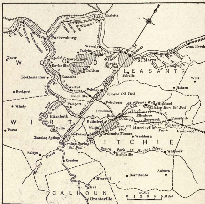
FIG. 47.—Map showing relation of grahamite fissure to anticlinal fold, in Ritchie County, W. Va. (After White, Bull. Geol. Soc. Amer. , X.)
