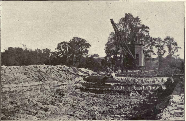
FIG. 2. — Marl pit at Warners, N. Y. The dark streaks are peat, and the marl is underlain by clay. ( H. Ries, photo. )
