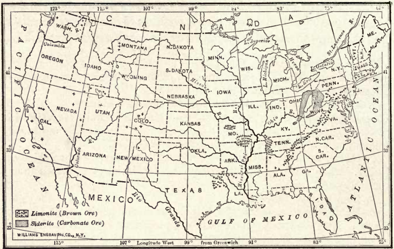
FIG. 174. — Map showing distribution of limonite and siderite in the United States. (After Harder.)
