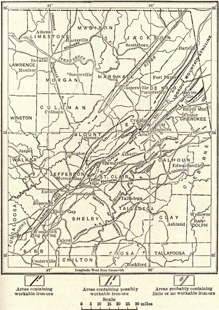
FIG. 170.— Map showing outcrop of Clinton ore in Alabama. (After Burchard, Amer. Inst. Min. Engrs., Bull. 24, 1908. )
