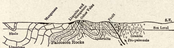
FIG. 272.—Section in Georgia manganese area, showing geologic relations of manganese, limonite, and ocher. (After Watson, Amer. Inst. Min. Engrs. Trans. XXXIV).
