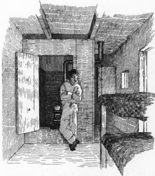
ARRANGEMENT OF QUARTERS ON TYPICAL EXPLOSIVES BARGE, SHOWING APPEARANCE OF METAL- AND ASBESTOS-LINED ROOM, WITH COAST GUARDSMAN INVARIABLY IN ATTENDANCE
