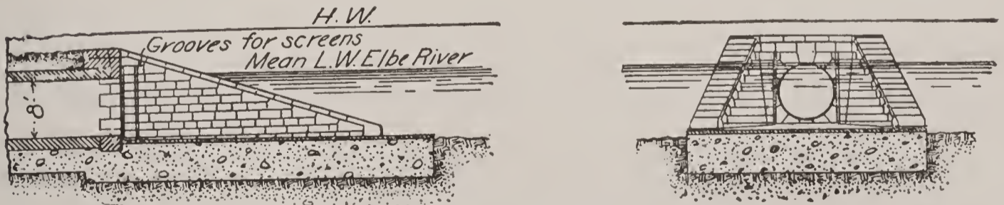
FIG. 40.—INTAKE AT HAMBURG, GERMANY.
