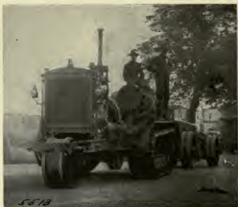
A 75 HOLT TRACTOR ON THE ROAD WITH A 155 G. P. F.
