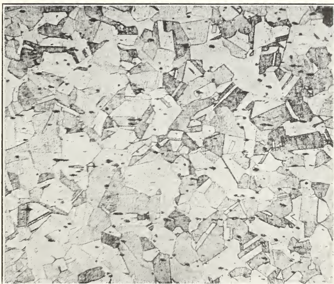
FIG. 2.—Microstructure of hot-rolled nickel rod. \times 100
