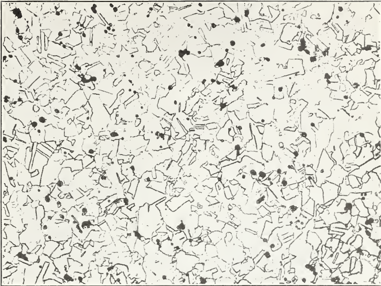
FIG. 15.—Microstructure of rolled Monel metal rod. \times 100
