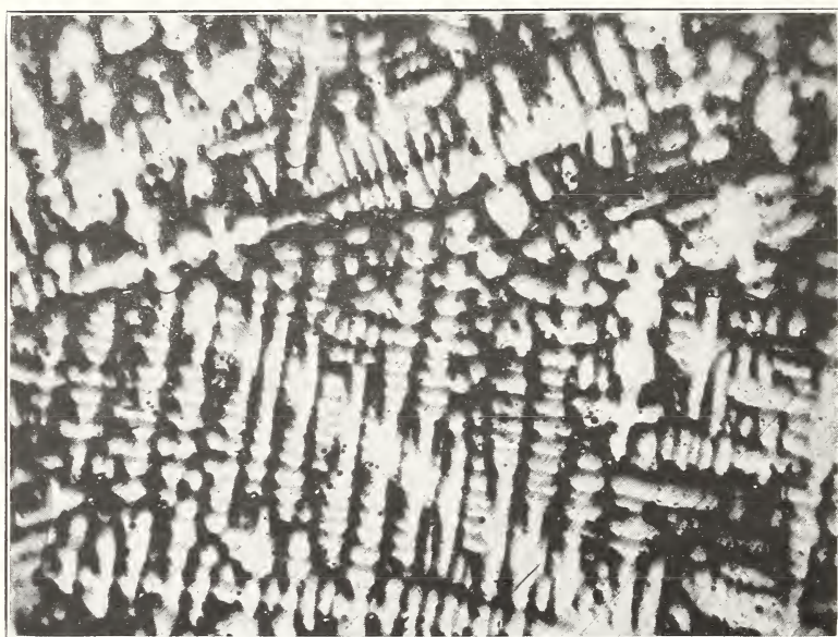
FIG. 17.— Microstructure of cast Monel metal. \times 100
