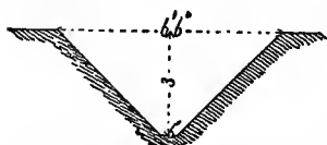
FIG. 2.—Cross-section of properly shaped ditch, three feet deep, six and one-half wide at the surface of the ground, six inches at the bottom.
