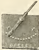
Fig. 1. Starting Panel of CR 130 Valve Controller.
