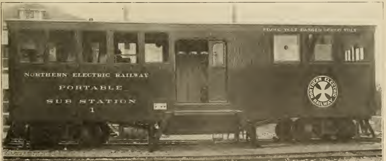
A Portable Sub-Station.
