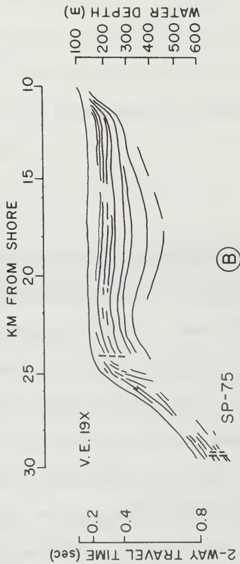
Figure 17. Sparker profiles across the southern Oregon shelf and upper slope. A. SP-47 (42°42'N). B. SP-75 (42°08'N). After Kulm and Fowler (1970).
