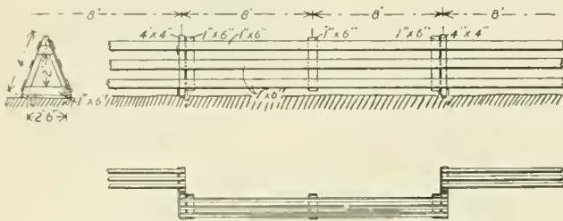
FIG. 1.—FENCE USED BY BOSTON ELEVATED.
