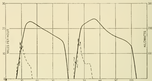
FIG. 10—ACCELERATION CURVES, CONTINUOUS CURRENT.
