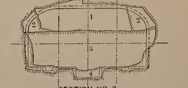
General Method of Excavation Adopted in the Bergen Hill Tunnels of the Pennsylvania R.R., entering New York.
