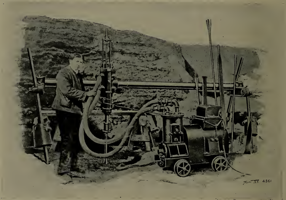
“Electric-Air” Rock Drill on Quarry Bar Mounting.
