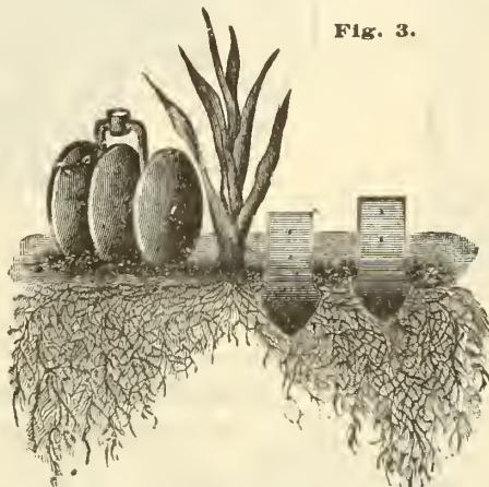
Diagram of a corn plant showing advantage of using the Janesville Disk Cultivator. Perfect tillage without injury to the roots of the young plants.
