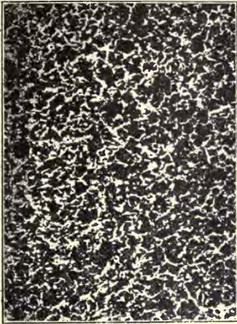
FIG. 258.—Normal Structure of .46 per cent Carbon Steel (Ferrite and Pearlite). V. 90 X.
