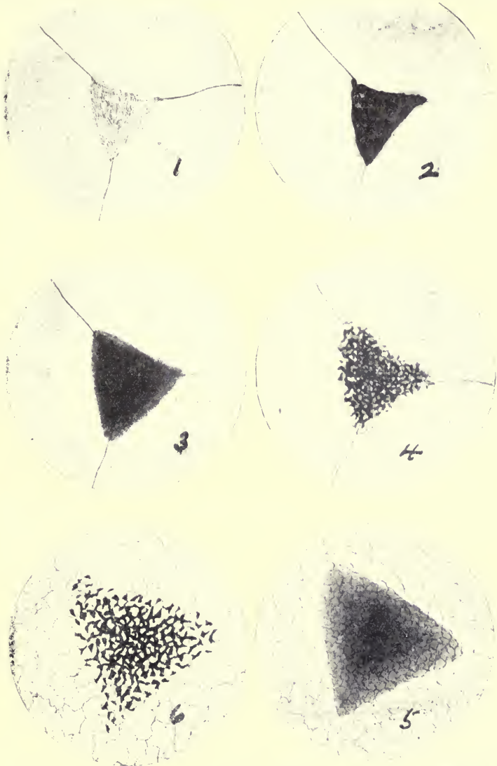
FIG. 262.—Diagram of changes which occur on heating, quenching, or slowly cooling a Mild Steel containing about 0.1 per cent Carbon. (Stead.)
