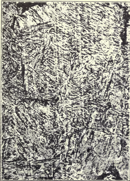
FIG. 226.—Martensite structure of .26 per cent Carbon Steel, quenched in water from 950 deg. Cen. after prolonged annealing. This shows some dark areas of Troostite and a small proportion of free Ferrite (white). Magnified 300 diameters.
