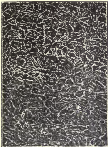
FIG. 254.—Normal Structure of 1.3 per cent Carbon Steel (Cementite and Pearlite). V. 90 X.
