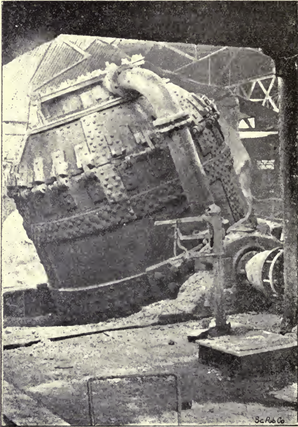
FIG. 129.—Bessemer Converter (Bottom up).
