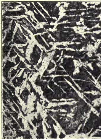
FIG. 260.—Overheated Structure of .46 per cent Carbon Steel (Ferrite and Pearlite lattice). V. 90 X.
