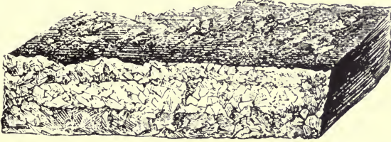
Fracture of Blister Steel.—Shear Heat.
