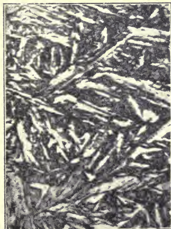
FIG. 256.—Martensitic Structure of 1.3 per cent Carbon Steel, quenched from 1,000 deg. Cen. (Austenite and Hardenite). V. 600 X
