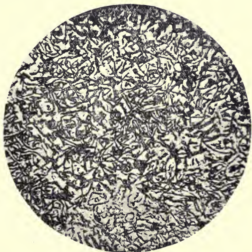
FIG. 250.—Eutectic Structure of Austenite and Graphite in 4.3 per cent Carbon iron slowly cooled from fusion and quenched at 1,000 deg. Cen. (Campbell.) Magnified 30 diameters.
