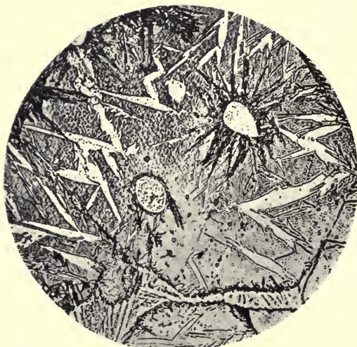
FIG. 252.—Austenite-Cementite Structure in the "Fusion Spots" of partially molten Steel (C. = 1.76 per cent) quenched in water at 1,170 deg. Cen. (Gutowsky.) Magnified 200 diameters.
