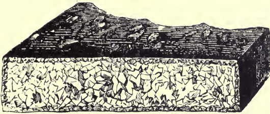
Fracture of Blister Steel.—Spring Heat.
