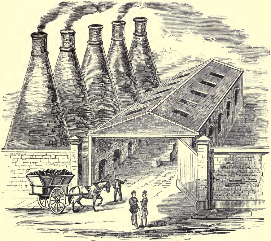
FIG. 113.—Steel Converting Furnaces.
