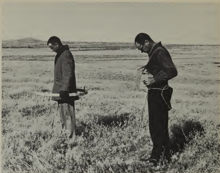
Geological Survey geophysicists searching in the field for buried ore bodies by means of the Slingram method. Electromagnetic waves, transmitted by a battery-powered portable antenna coil, out of view to the right, are received by coil on the left; ratiometer and amplifier unit, shown on the right, compare the received signal with the transmitted signal, showing disturbances of the electromagnetic field which could be caused by a buried, electrically conductive ore body.
