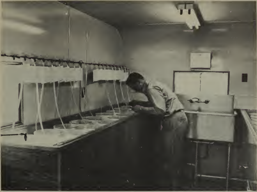
Mobile bioassay laboratory in which streamside tests are made to determine exact amounts of selective chemical toxicant that will kill sea lamprey larvae but not other species of fish.
