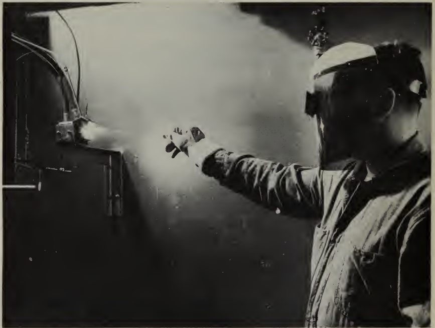
In research on obtaining new or improved products from one of the Nation's most abundant resources, Bureau scientists are reacting coal at extremely high temperatures in this "plasma jet" unit . . .
