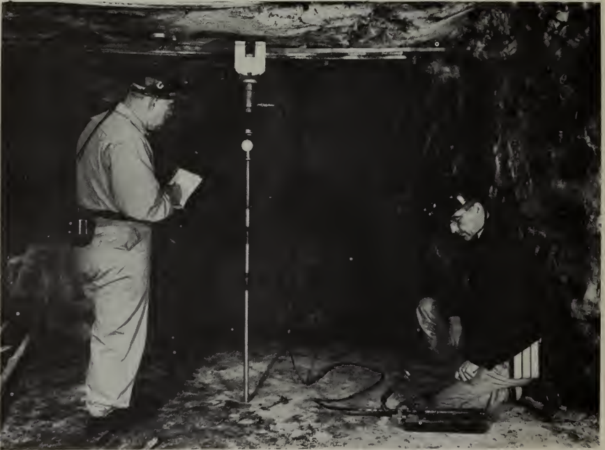
Bureau of Mines engineers test a device newly developed by the Bureau for determining whether roof bolts are securely anchored in the layers of earth and rock they are designed to support.
