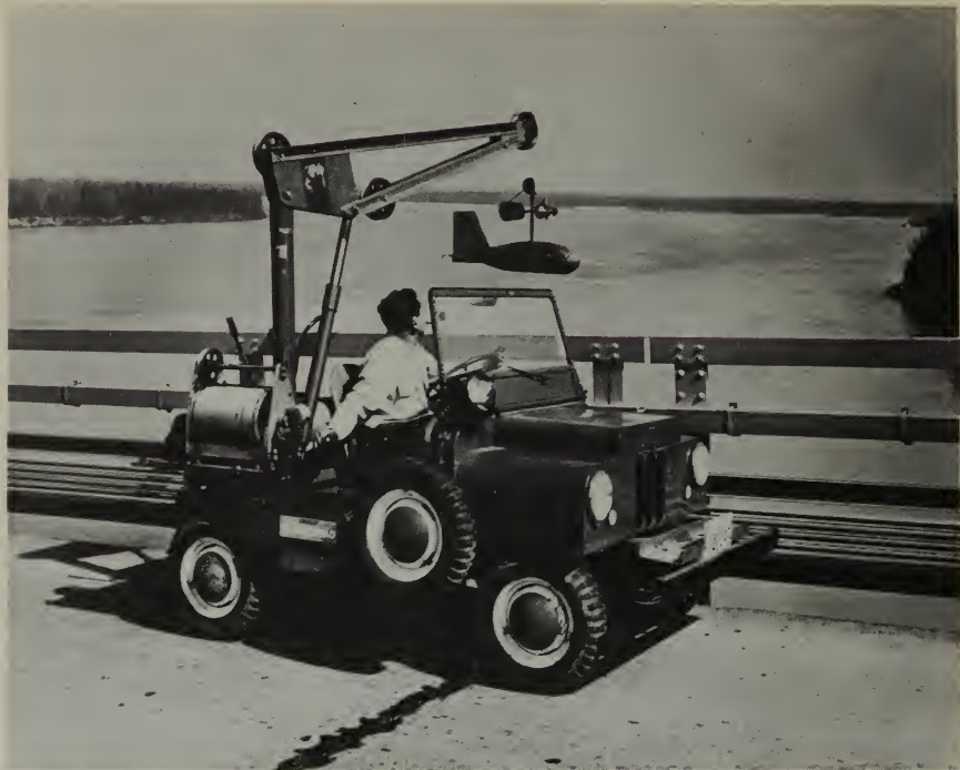
A Geological Survey engineer uses a jeep-mounted crane with sounding weight and current meter to measure the flow of the Mississippi River at Vicksburg, Miss.
