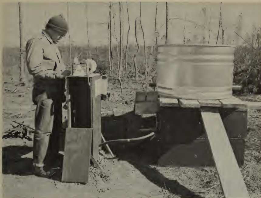
A Geological Survey engineer determines the transmissibility of an aquifer in the Piedmont Province in Georgia by feeding water into a well at a constant rate and observing the change in water surface elevation.
