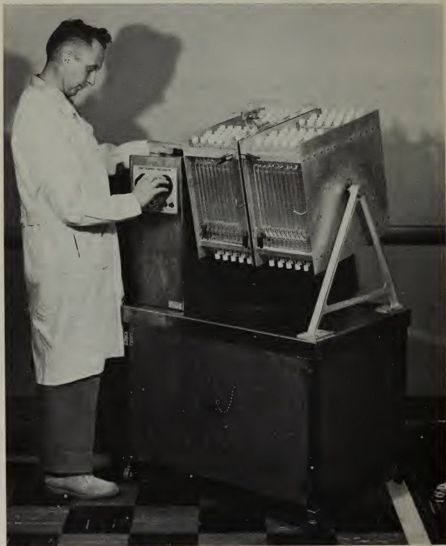
Different components of shale oil are separated from one another in this apparatus at a Bureau of Mines research center.
