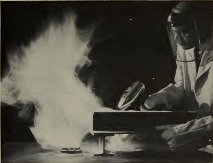
Using a small blower device, a Bureau of Mines scientist dispenses a cloud of cellulose acetate dust over a lighted candle, demonstrating one of the hazards encountered in handling combustible industrial materials.
