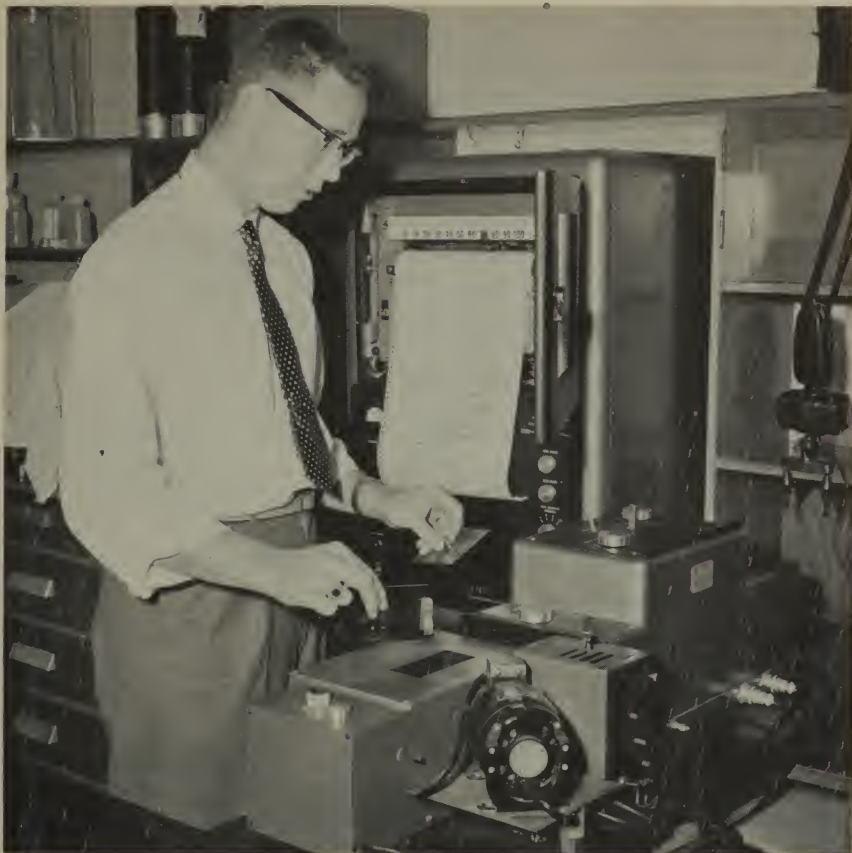
Ultraviolet recording spectrophotometer being used for chemical studies on fish oils.
