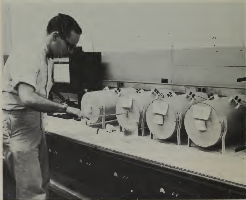
Geological Survey geologist quenches an experimental sulfide mineral batch for studies in environment of ore deposition.
