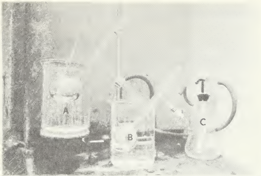
Fig.6. Vacuum evaporation apparatus for the reduction of the sample volume: (A) 35°C oil bath containing glass bulb for sample, (B) ice bath containing glass bulb for evaporated solvent, and (C) vacuum aspirator safety bottle.
