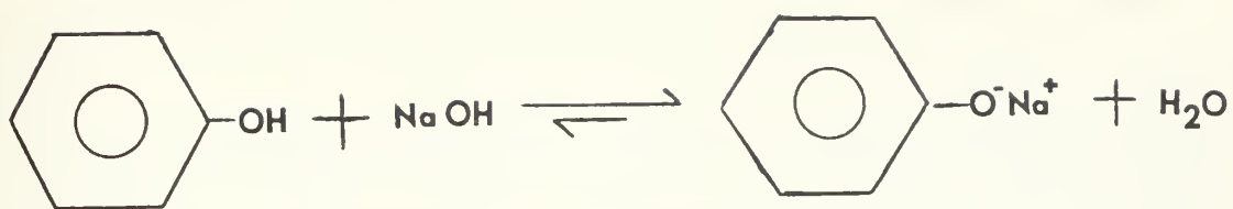
Fig. 45. Phenol Conjugate Acid, Base Reaction
