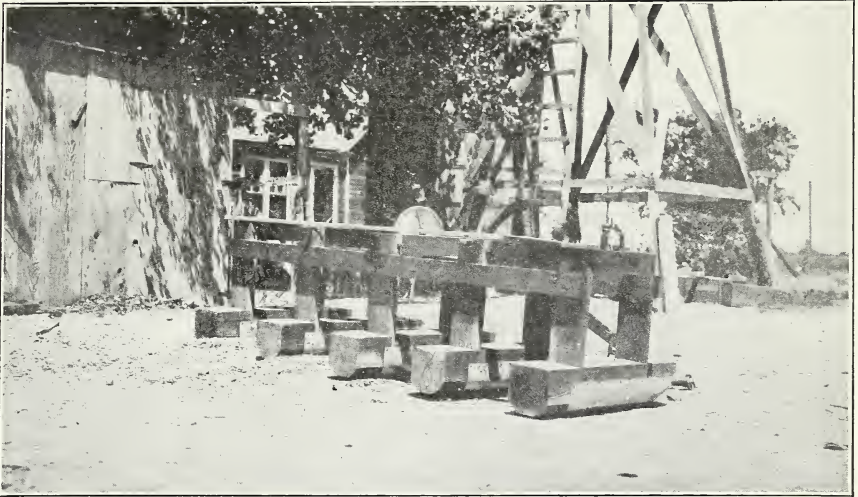
FIG. 1.—A SLEDGING IMPLEMENT USED IN SMOOTHING IRRIGATING FURROWS IN SUGAR-BEET FIELDS, BEING SOMETIMES HELPFUL IN DISTRIBUTING THE WATER.
