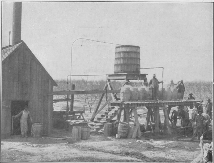
FIG. 2.—A WELL-ARRANGED PLANT FOR COOKING THE WASH ON A LARGE SCALE. (AFTER R. I. SMITH.)
