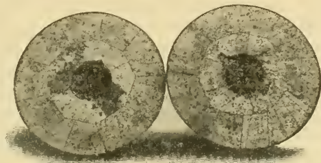
A pair of burr stones, used before the advent of steel rolls.
