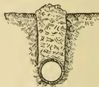
A modern tile drain.
