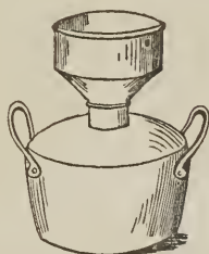
Water bath for drying filters.
