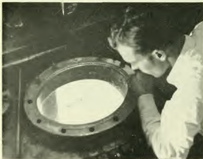
2. BATCH OF CRUDE METHYL METHACRYLATE POLYMER, THE BASE FOR "LUCITE" PLASTIC MANUFACTURED BY E. I. DU PONT DE NEMOURS & CO. AT THE COMPANY'S BELLE, W. VA., PLANT.
