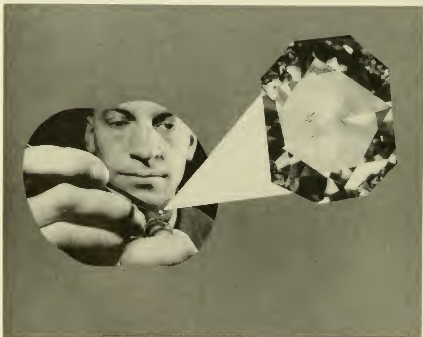
2. Face of natural diamond gem stone (right) scratched by a piece of Borazon.
