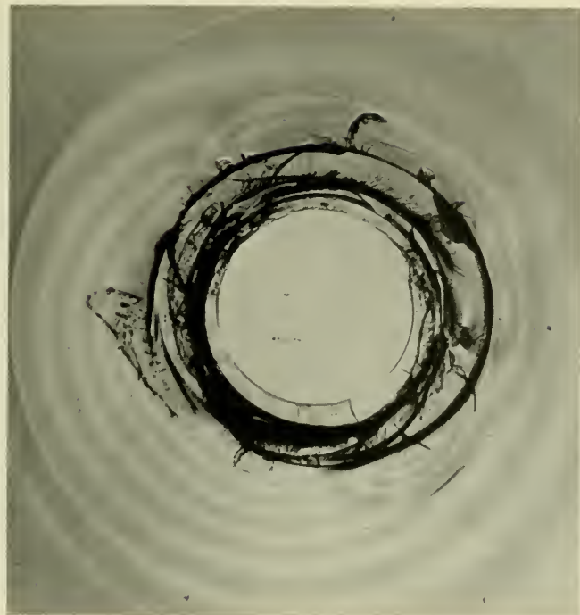
2. A ring fracture produced by pressing a \frac{1}{2} inch diameter steel ball against plate glass. (Magnification \times 23 .)
