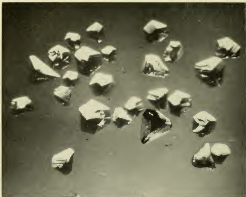
1. Borazon—a completely new material never found in nature (56 X).
