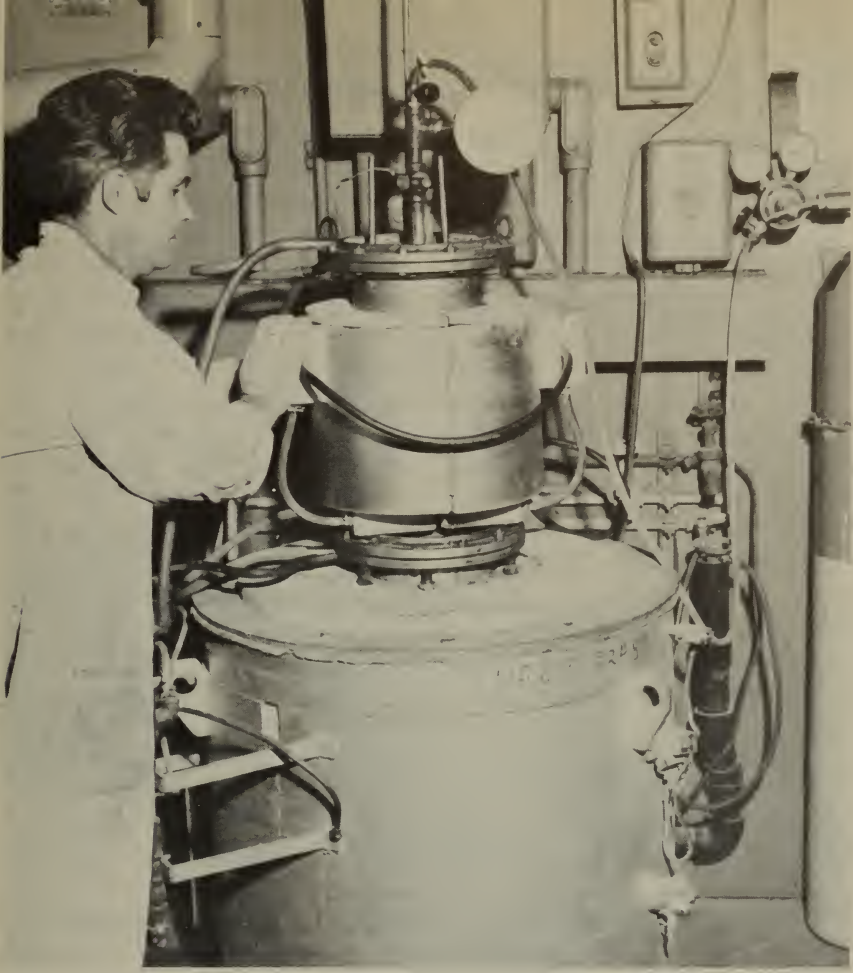
As part of its metallurgical research, the Bureau of Mines operates this experimental retort for producing tantalum or columbium by the Kroll process.
