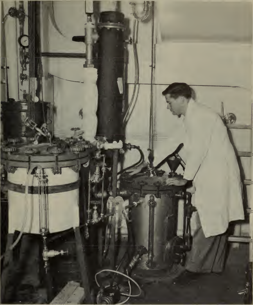
Extraction of oil from tuna meal preparatory to evaluating the protein quality of the meal as chick feed component.
