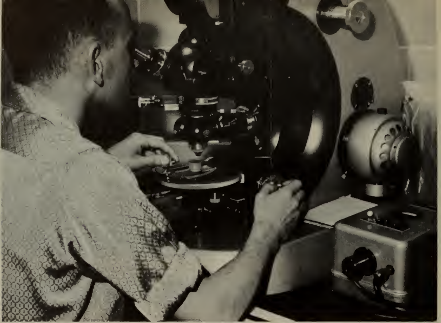
Mineralogists and petrologists use this ultraphoto microscope for examining mineral specimens at the Bureau of Mines' new research station, Fort Snelling, Minn.
