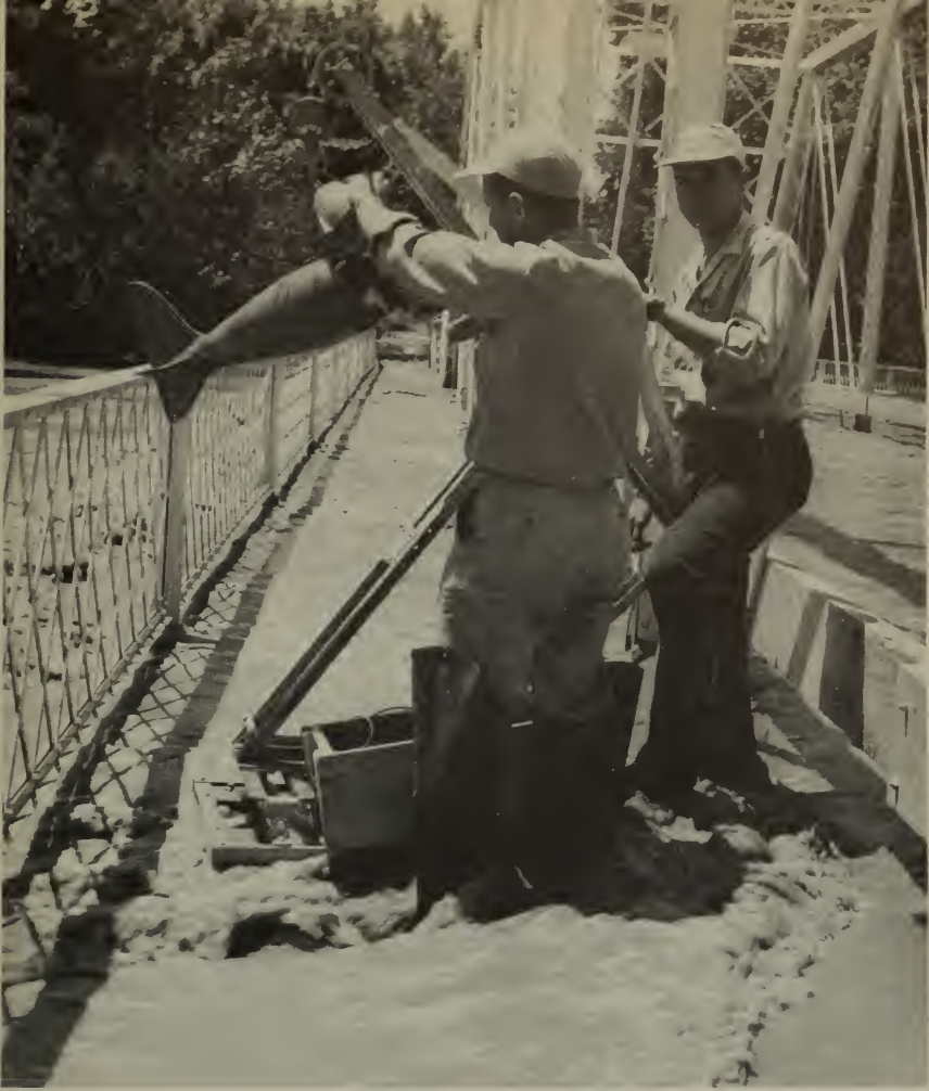
Sampling the sediment load of the Solomon River at Beloit, Kansas during a flood.
