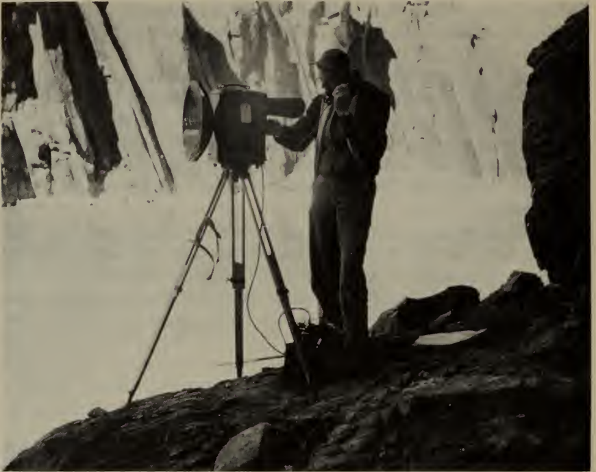
Electronic surveying has replaced the miles of weary walking to measure distances. Deep in Colorado's Glen Canyon this surveyor will move by helicopter to his next station.
