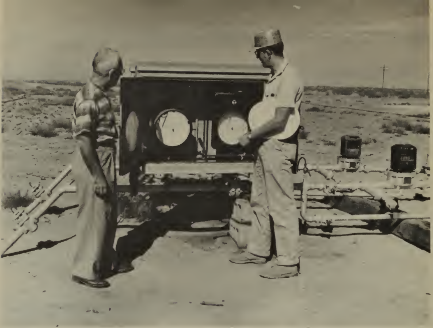
Survey petroleum engineer, accompanied by operator's representative, checking temperature and volume of butane going from lease to storage. On-site inspections assure resource conservation and protection of the Government's royalty interest.
