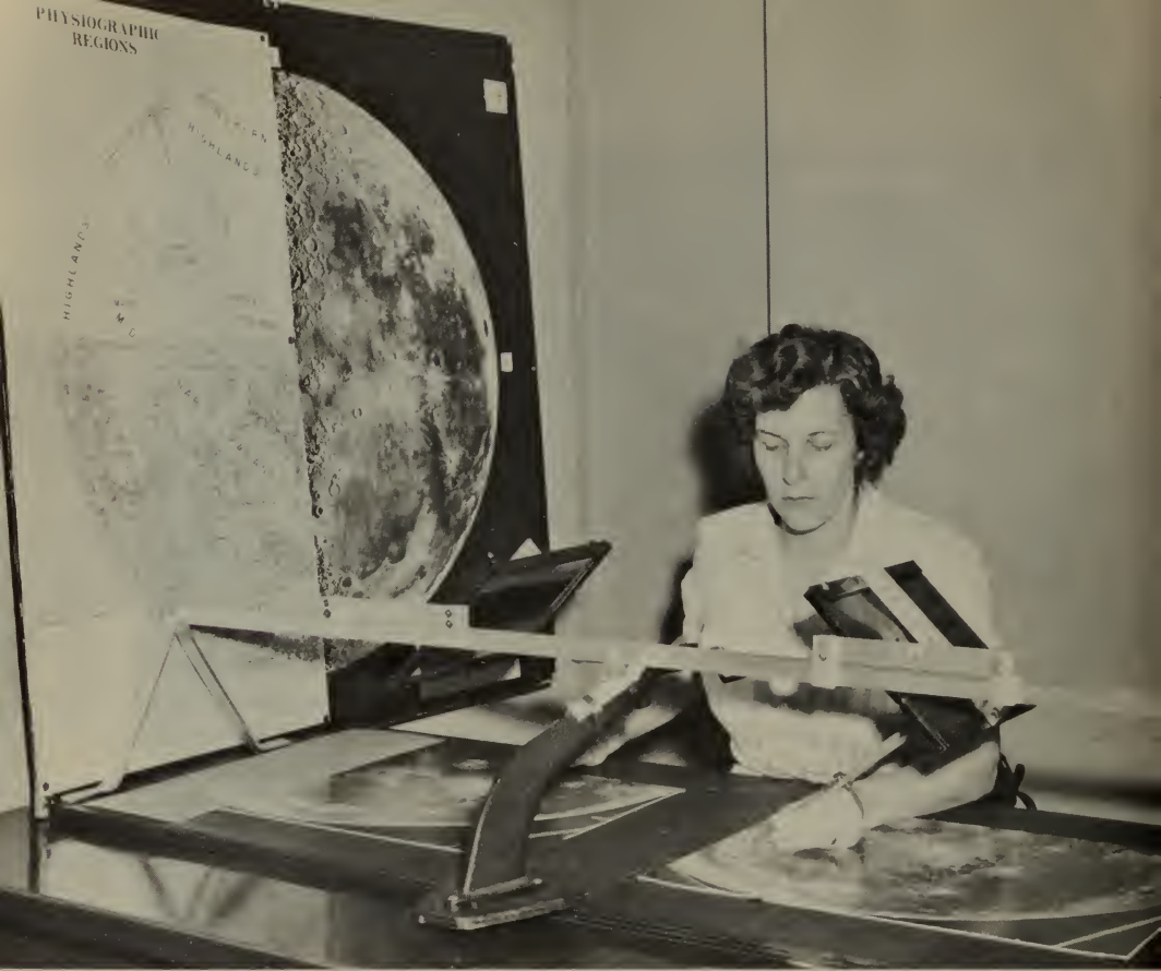
Photogeologist measuring the diameter of a crater on the spherical surface of the moon. Using stereoscopic photoviewer, the geologic features of the moon's surface are carefully diagrammed to produce detailed maps.
