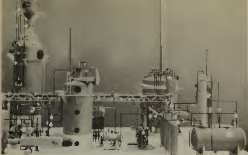
Model of 35,000 GPD freezing process pilot plant being built at St. Petersburg, Fla.
