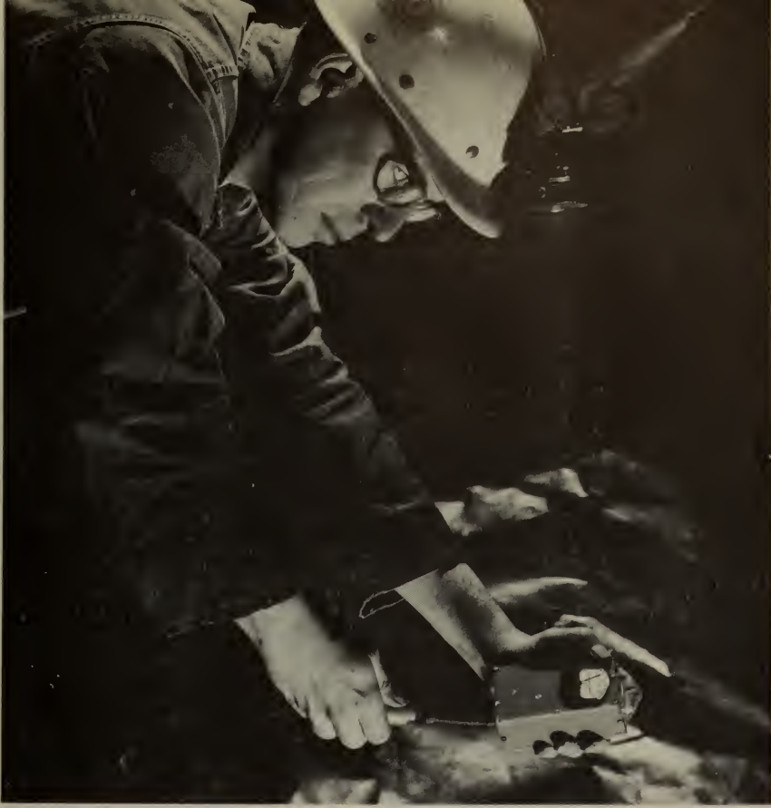
A new device for detecting combustible gases, developed by the Bureau of Mines, is demonstrated here in an underground mine.
