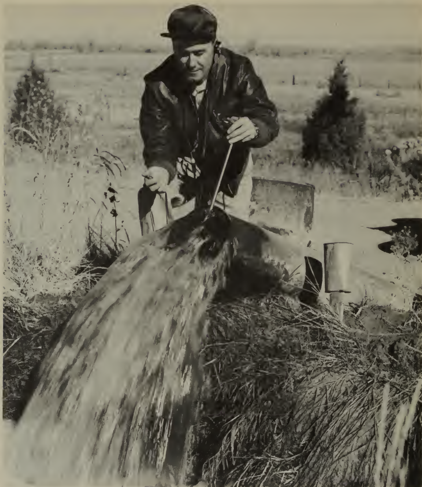
A Geological Survey ground water engineer measuring flow of water from pump discharge pipe as part of a nationwide inventory of the country's ground-water resources.
