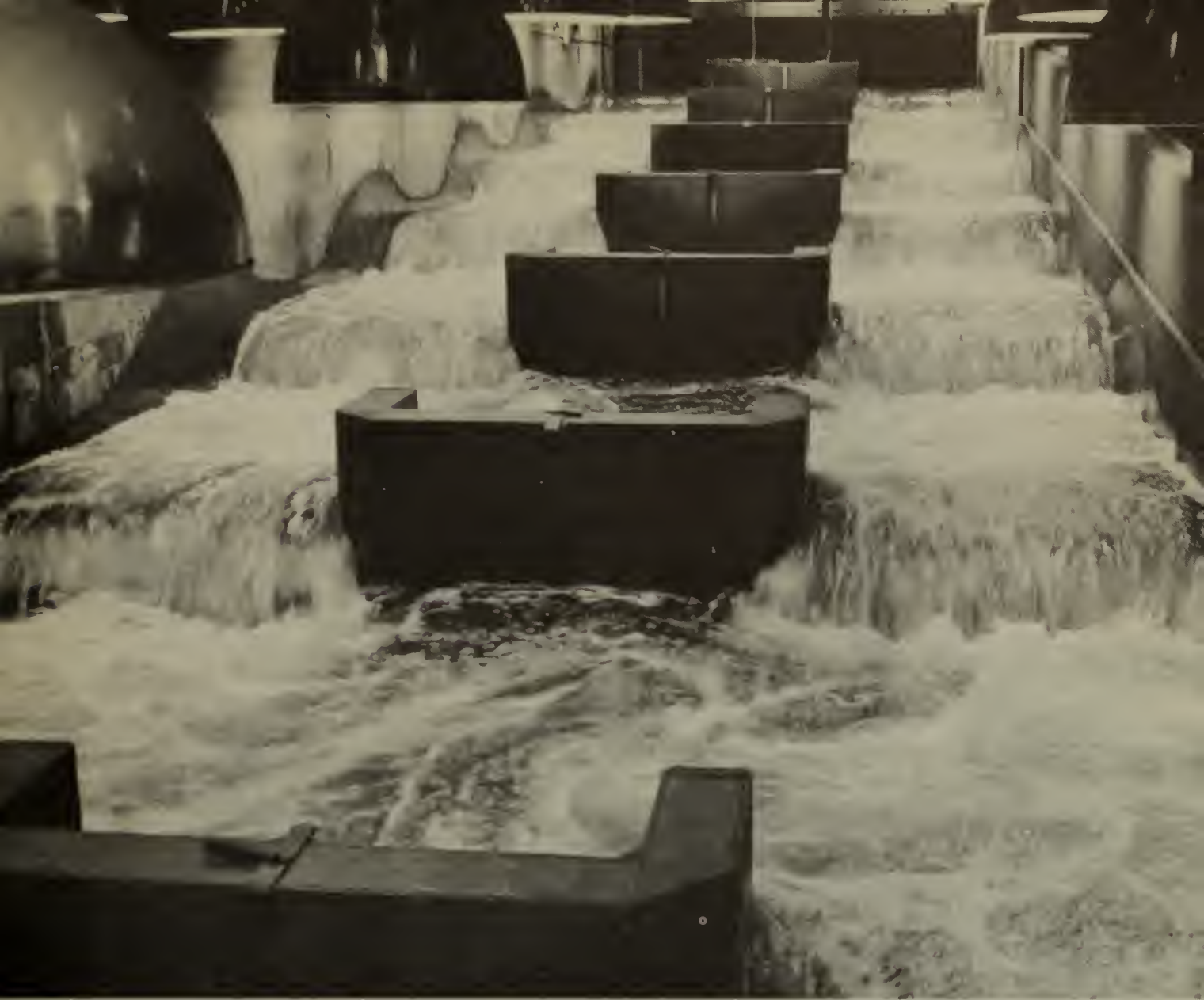
Testing the 6-pool prototype of the fishway designed for Ice Harbor Dam. The "steps" in this "stairway" are 1 foot high and 10 feet long.
