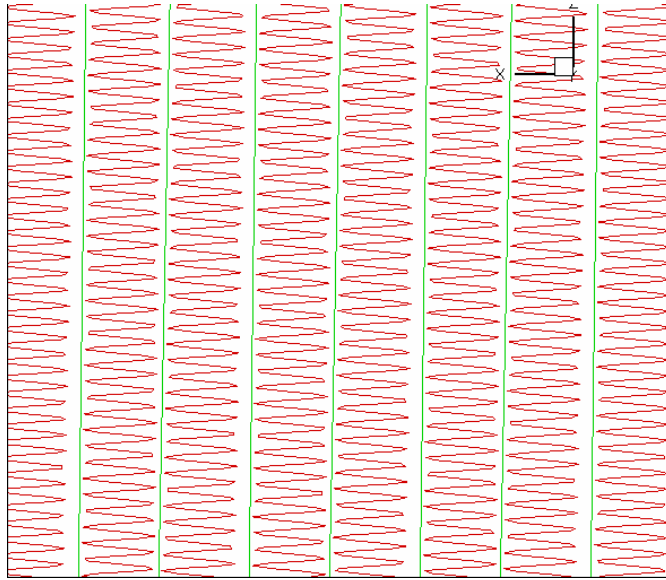
Figure 3.6.4: The bottom figure from Figure 3.6.1. This is the center of the comparisons of the trajectories. Note that the guiding center is always to the left of the Boris trajectory. This is based on the same starting point for each simulation. The electron actually spirals around the field lines and the guiding center ignores the spiral and just follows the general motion of the guiding center.
