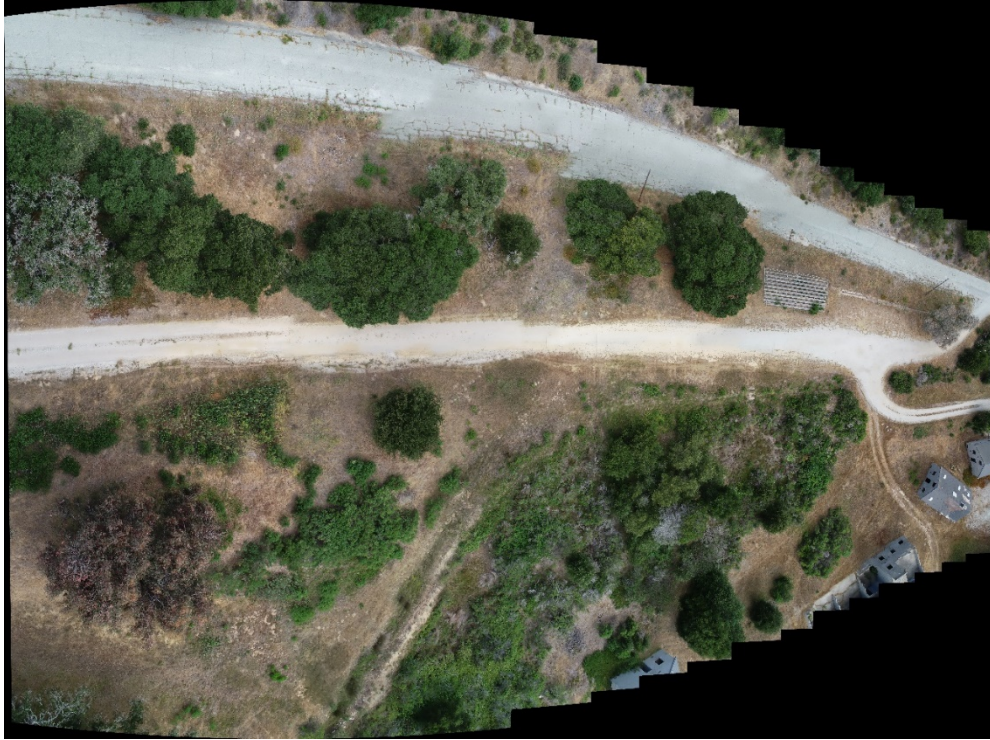
Figure 32. Mosaic showing vanishing effect due to UAV flight parameter settings.
