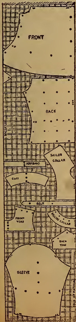
The Most Economical Way of Placing the Pieces of Pattern No. 1039 on Forty-Four-Inch Material
