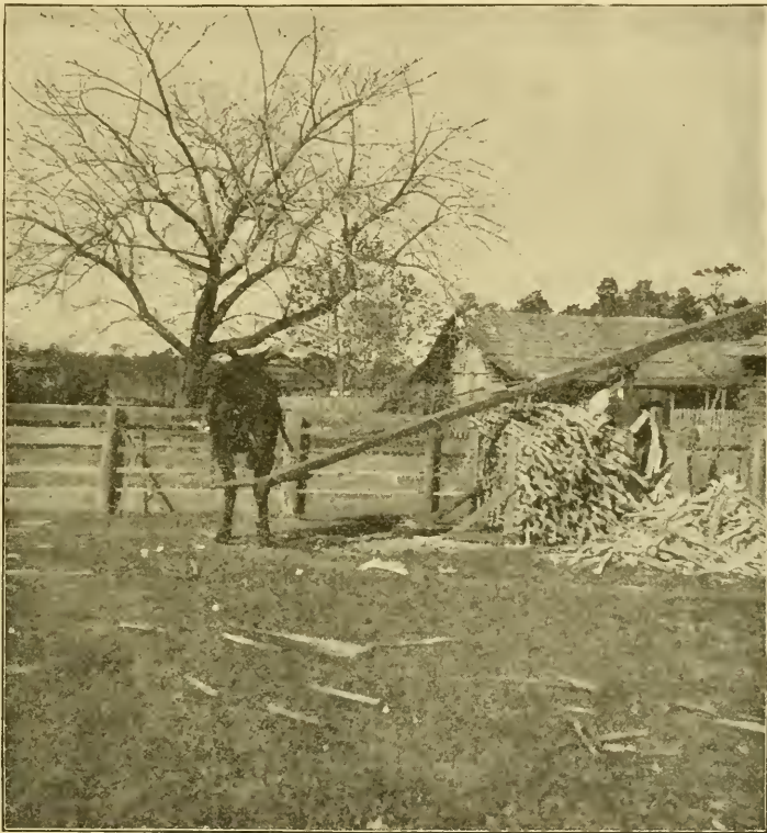
FIG. 80.—SMALL PRIMITIVE MILL FOR EXTRACTING JUICE FROM SUGAR CANE FOR SIRUP MAKING. —(Photograph by H. W. Wiley.)
