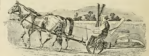
FIG. 9.—A modern self-rake reaper.
