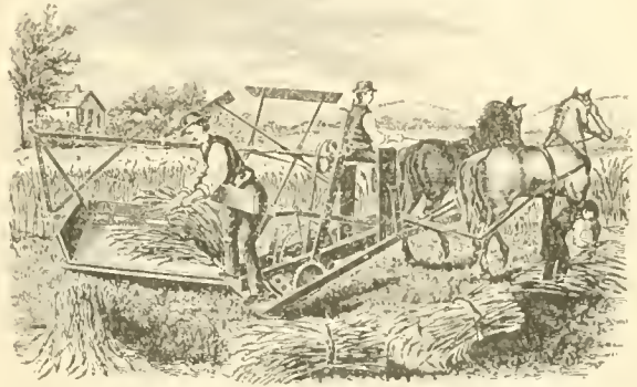
FIG. 4.—The McCormick reaper of 1845. The raker is carried on the machine.
