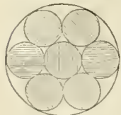
FIG. 4.—A single strand of a 49-wire rope.
